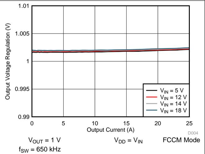
Figure 4. Output Voltage Regulation vs Output Current
