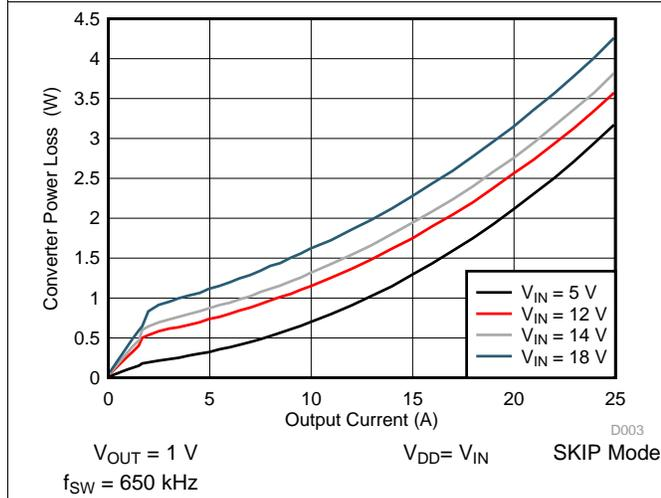
Figure 3. Converter Power Loss vs Output Current
