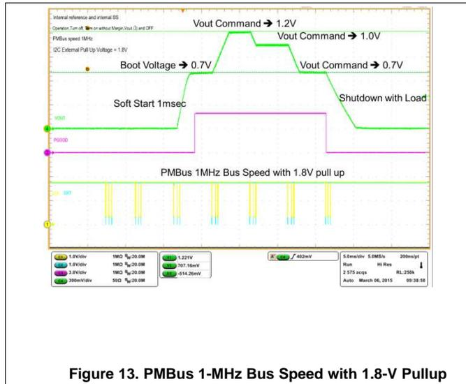
Figure 13. PMBus 1-MHz Bus Speed with 1.8-V Pullup
