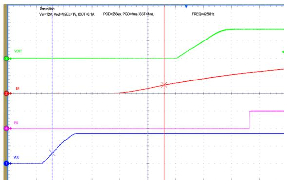
**Figure 27. Proper Sequencing of V<sub>DD</sub> and EN\_UVLO to Support the use of 4-ms SS Setting**
