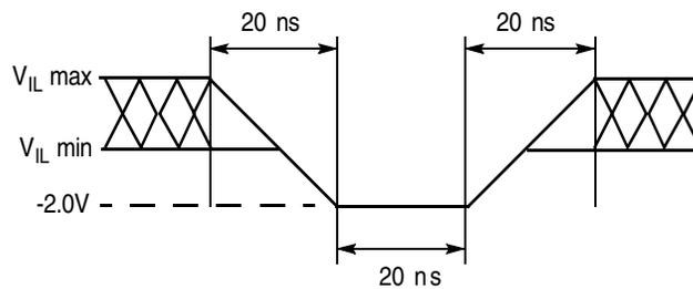
Figure 12. Maximum Positive Overshoot Waveform
