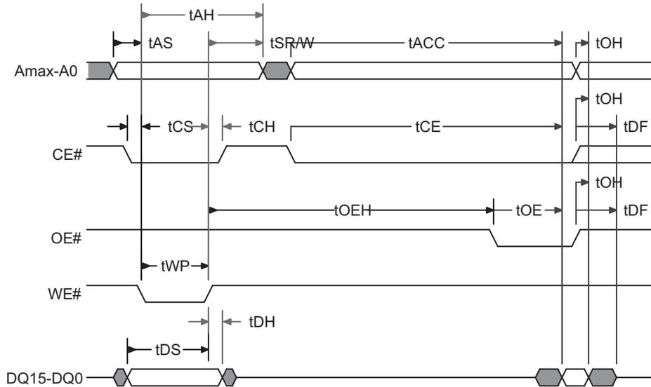
Figure 24. Read to Write ( $CE\# V_{IL}$ ) Operation Timing Diagram<sup>[155]</sup>
