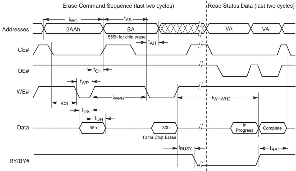
Figure 29. Data# Polling Timing Diagram (During Embedded Algorithms)<sup>[164]</sup>
