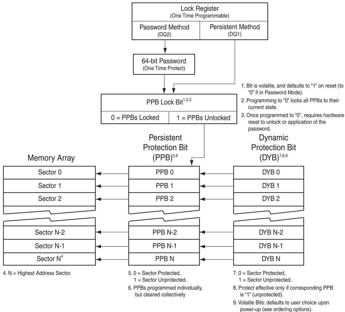
Every main flash array sector has a non-volatile (PPB) and a volatile (DYB) protection bit associated with it. When either bit is 0, the sector is protected from program and erase operations.
