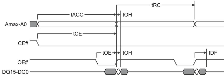
**Figure 19. Page Read Timing Diagram<sup>[149, 151]</sup>**
