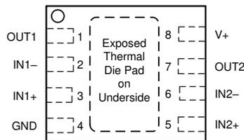
NOTE: Connect exposed thermal pad directly to GND pin.
