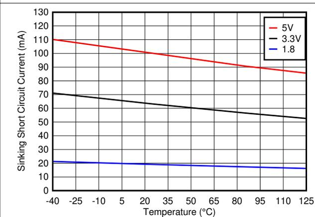
Figure 6-10. Sinking Short Circuit Current vs. Temperature
