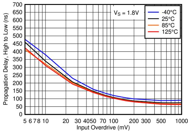
**Figure 6-13. Propagation Delay, High to Low, 1.8V**
