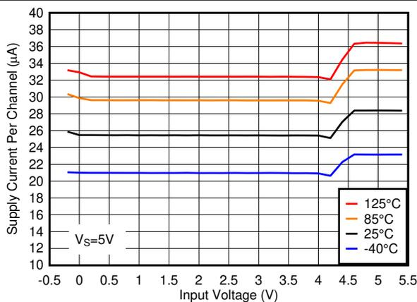
Figure 6-5. Supply Current vs. Input Voltage, 5V
