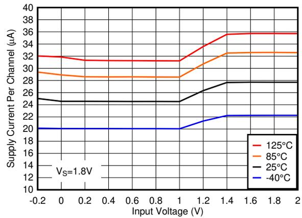
Figure 6-3. Supply Current vs. Input Voltage, 1.8V
