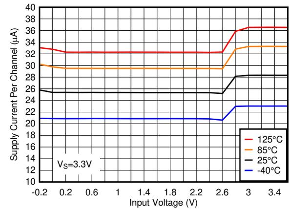
Figure 6-4. Supply Current vs. Input Voltage, 3.3V
