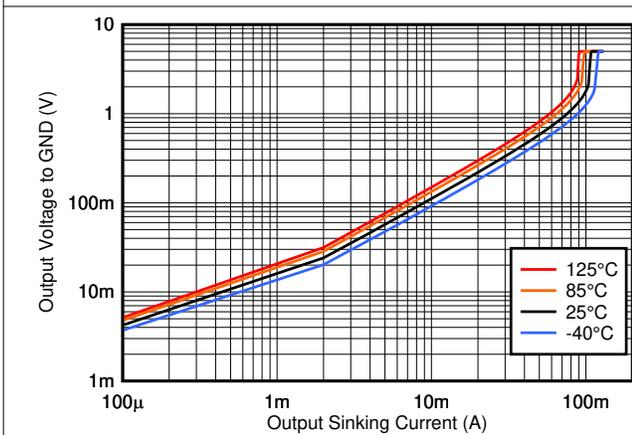
Figure 6-9. Output Sinking Current vs. Output Voltage, 5V
