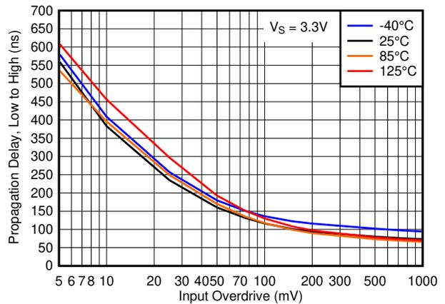
**Figure 6-16. Propagation Delay, Low to High, 3.3V**
