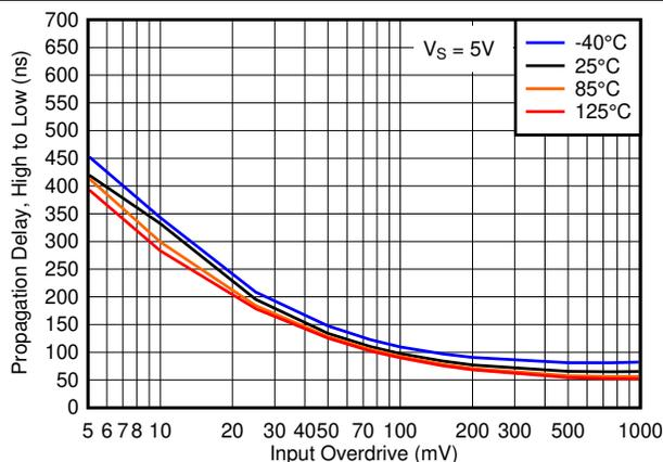
**Figure 6-17. Propagation Delay, High to Low, 5V**
