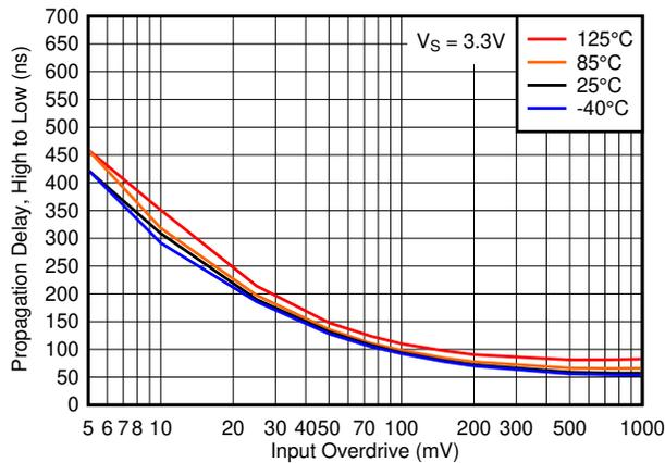
**Figure 6-15. Propagation Delay, High to Low, 3.3V**
