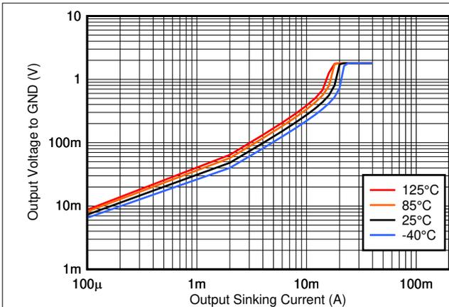
Figure 6-7. Output Sinking Current vs. Output Voltage, 1.8V
