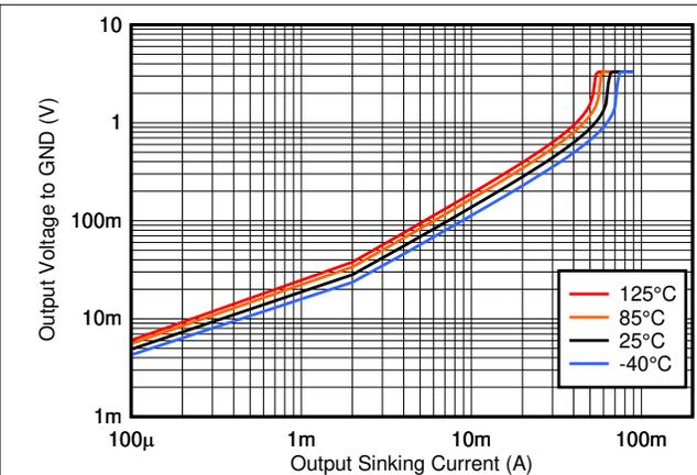
Figure 6-8. Output Sinking Current vs. Output Voltage, 3.3V
