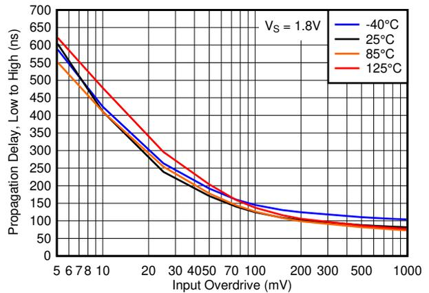
**Figure 6-14. Propagation Delay, Low to High, 1.8V**
