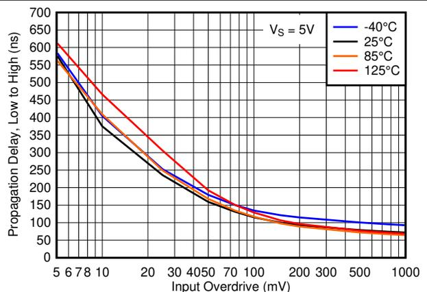
**Figure 6-18. Propagation Delay, Low to High, 5V**
