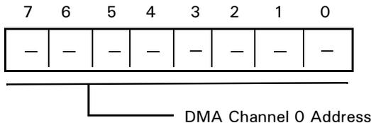
Figure 56. DMA Source Address Register 0 High
