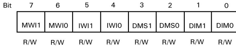
Figure 73. DMA/WAIT Control Register (DCNTL: I/O Address = 32H)
