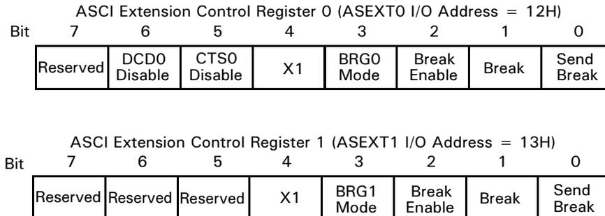
**Figure 47. ASCII Extension Control Registers, Channels 0 and 1**
