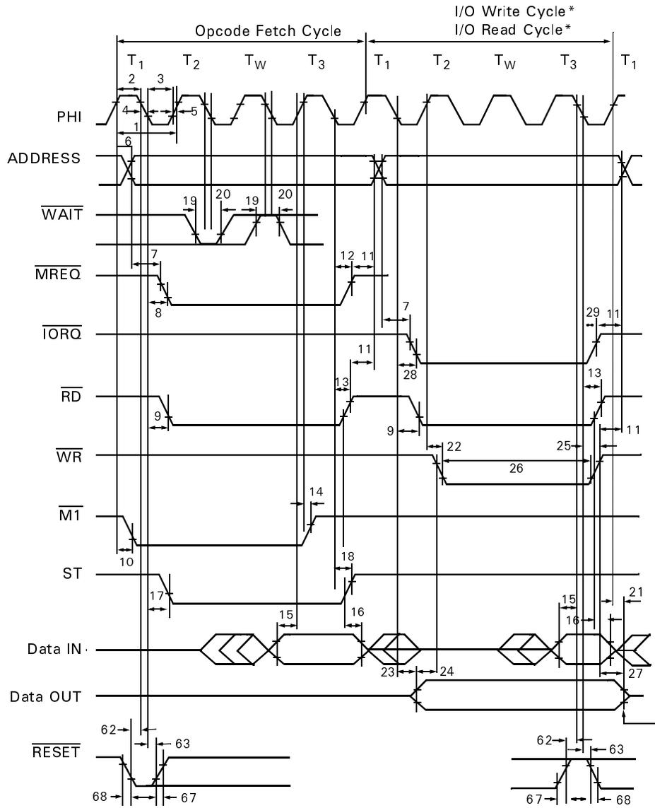
Note: \*Memory Read/Write Cycle timing is the same as I/O Read/Write Cycle except there are no automatic wait states (T<sub>W</sub>), and MREQ is active instead of IORQ.
