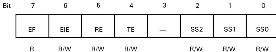
Figure 40. CSI/O Control Register (CNTR: I/O Address = 000AH)
