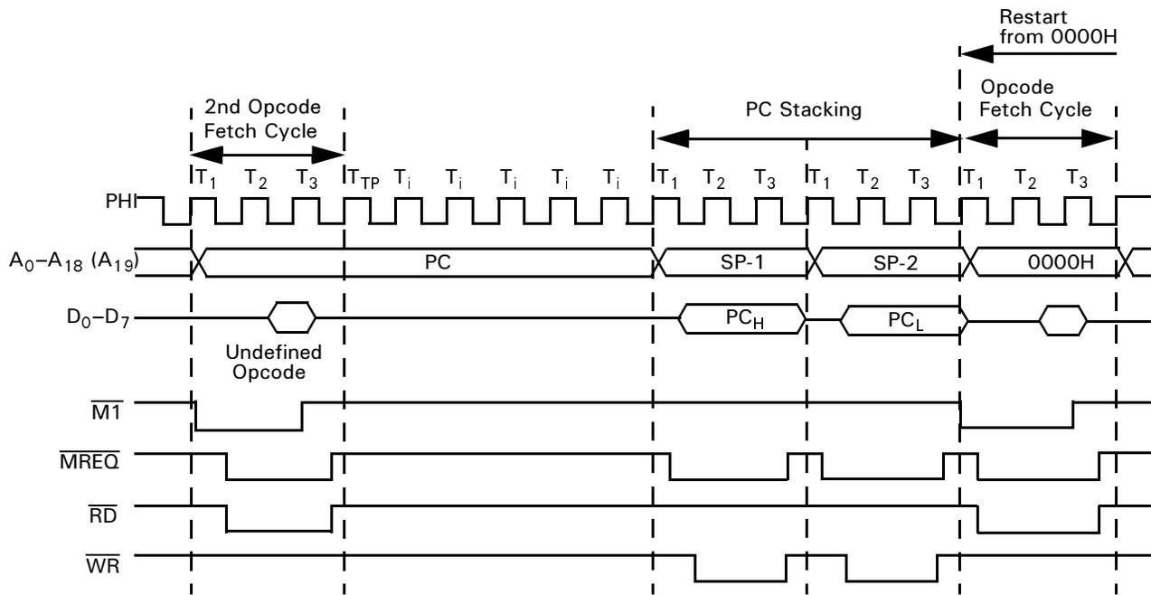
Figure 75. TRAP Timing—2<sup>nd</sup> Opcode Undefined
