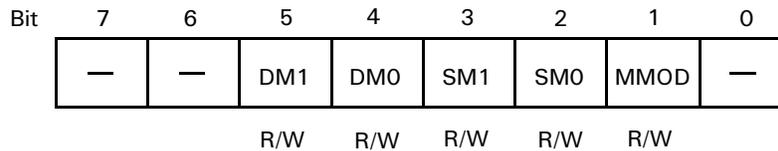
**Figure 72. DMA Mode Register (DMODE: I/O Address = 31H)**
