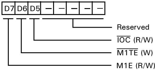
**Figure 8. Operating Control Register (OMCR: I/O Address = 3EH)**
