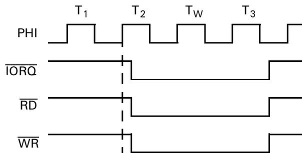
Figure 12. I/O Read and Write Cycles with  $\overline{IOC} = 0$
