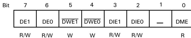
Figure 71. DMA Status Register (DSTAT: I/O Address = 30H)
