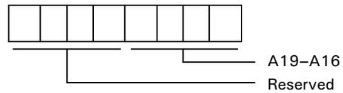
Figure 67. DMA Memory Address Register, Channel 1B
