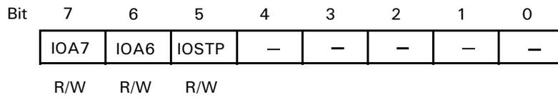
**Figure 83. I/O Control Register (ICR: I/O Address = 3FH)**
