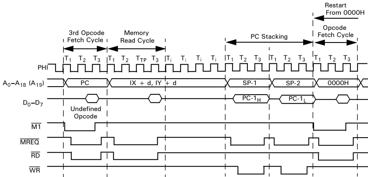
Figure 76. TRAP Timing—3<sup>rd</sup> Opcode Undefined
