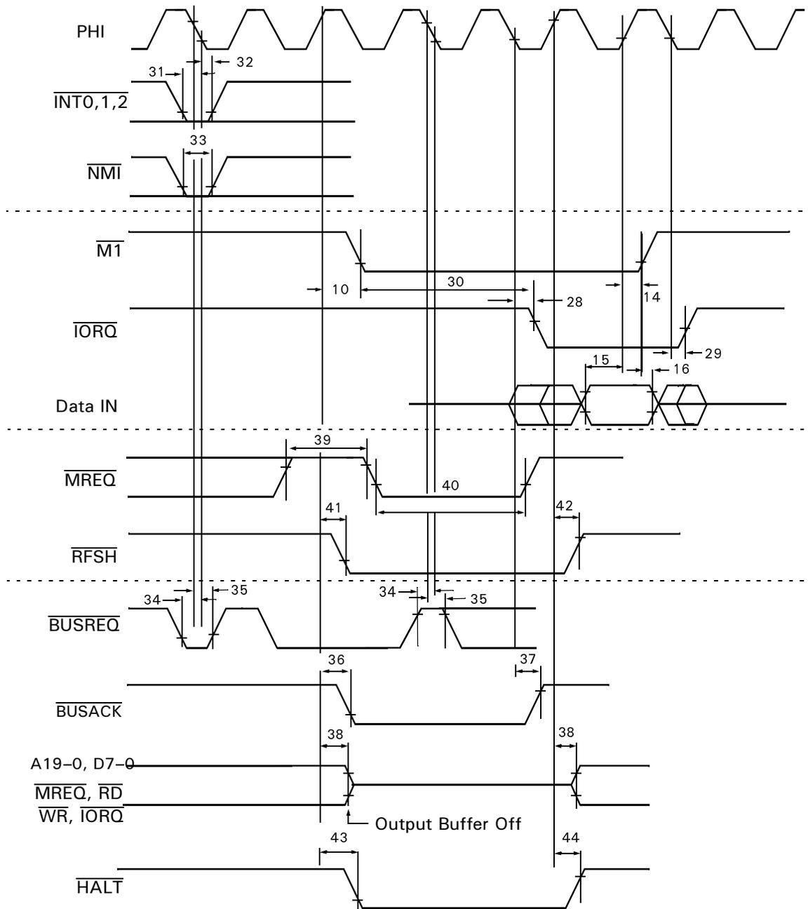
**Figure 21. CPU Timing**
