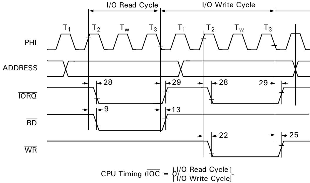
Figure 22. CPU Timing ( $\overline{\text{IOC}} = 0$ )
