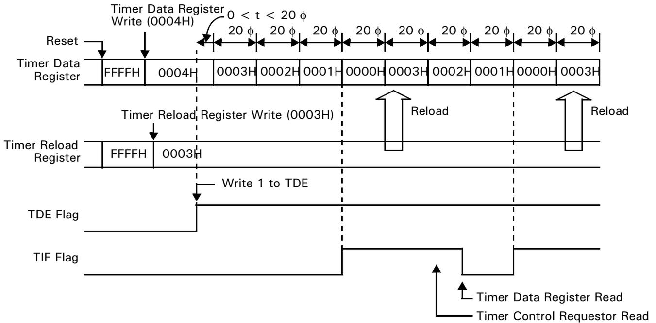
Figure 5. Timer Initialization, Count Down, and Reload Timing
