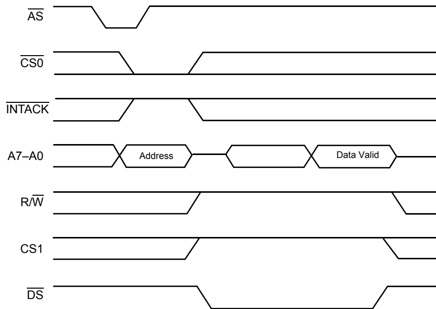
Figure 18. Z80230 Read Cycle Timing
