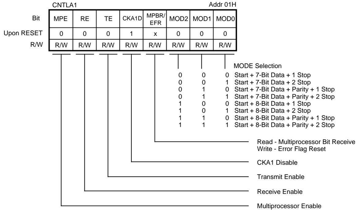
**Figure 10b. ASCII Control Register A** (Ch. 1)
