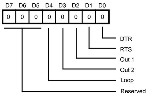
**Figure 77. Modem Control Register**
