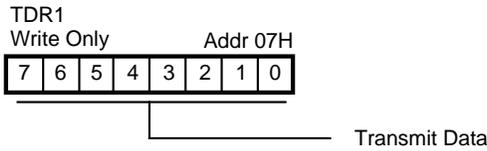
Figure 16. ASCII Transmit Data Register (Ch. 1)
