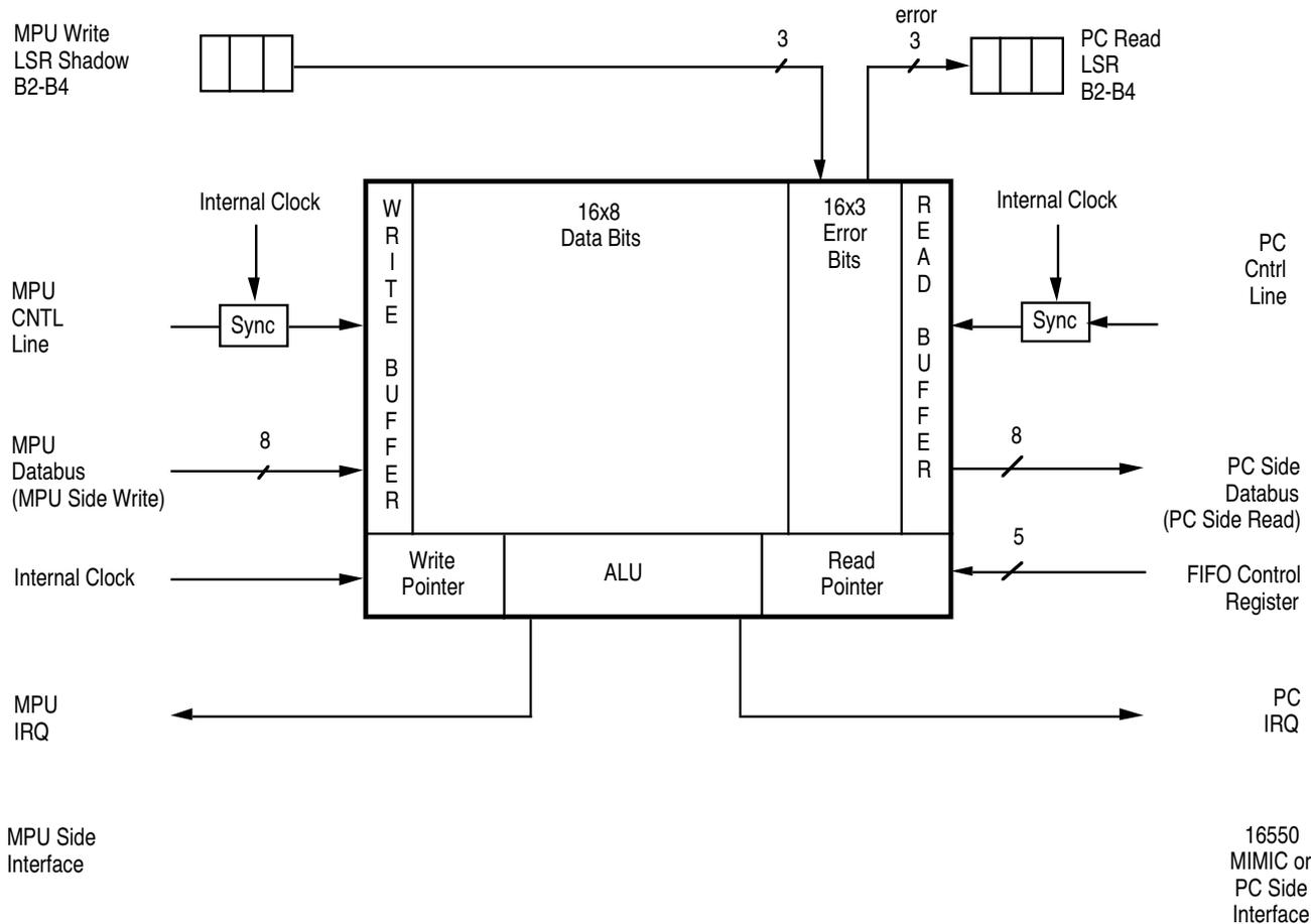
Figure 7. 16550 MIMIC Receiver FIFO Block Diagram
