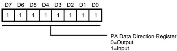
**Figure 83. PA, Port A, Data Direction Register**
