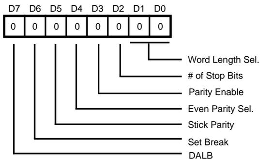
**Figure 76. Line Control Register**
