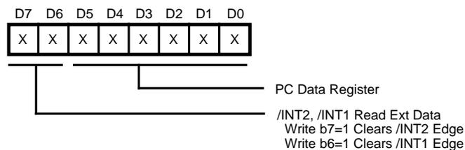
**Figure 88. PC, Port C, Data Register**
