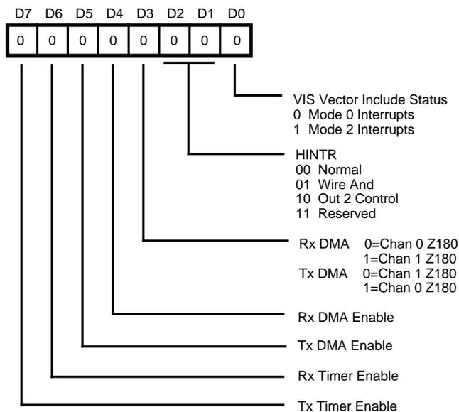
**Figure 60. MIMIC Master Control Register**
