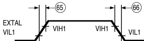
**Figure 102. External Clock Rise Time and Fall Time**
