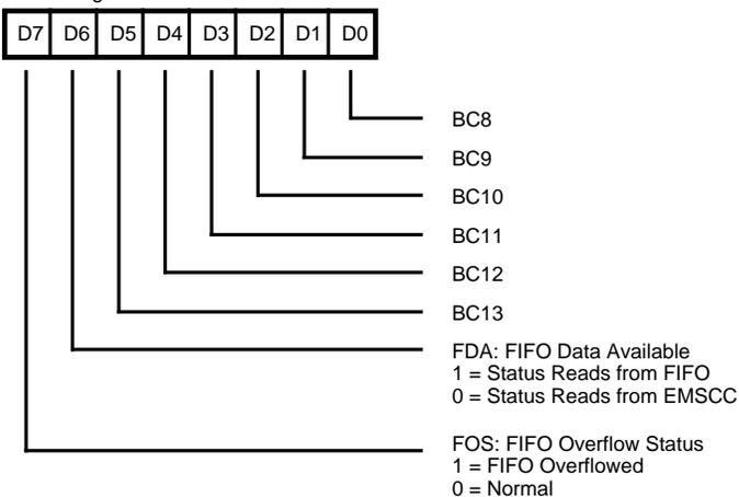
\*Can only be accessed if the SDLC FIFO enhancement is enabled (WR15 bit D2 set to 1)
