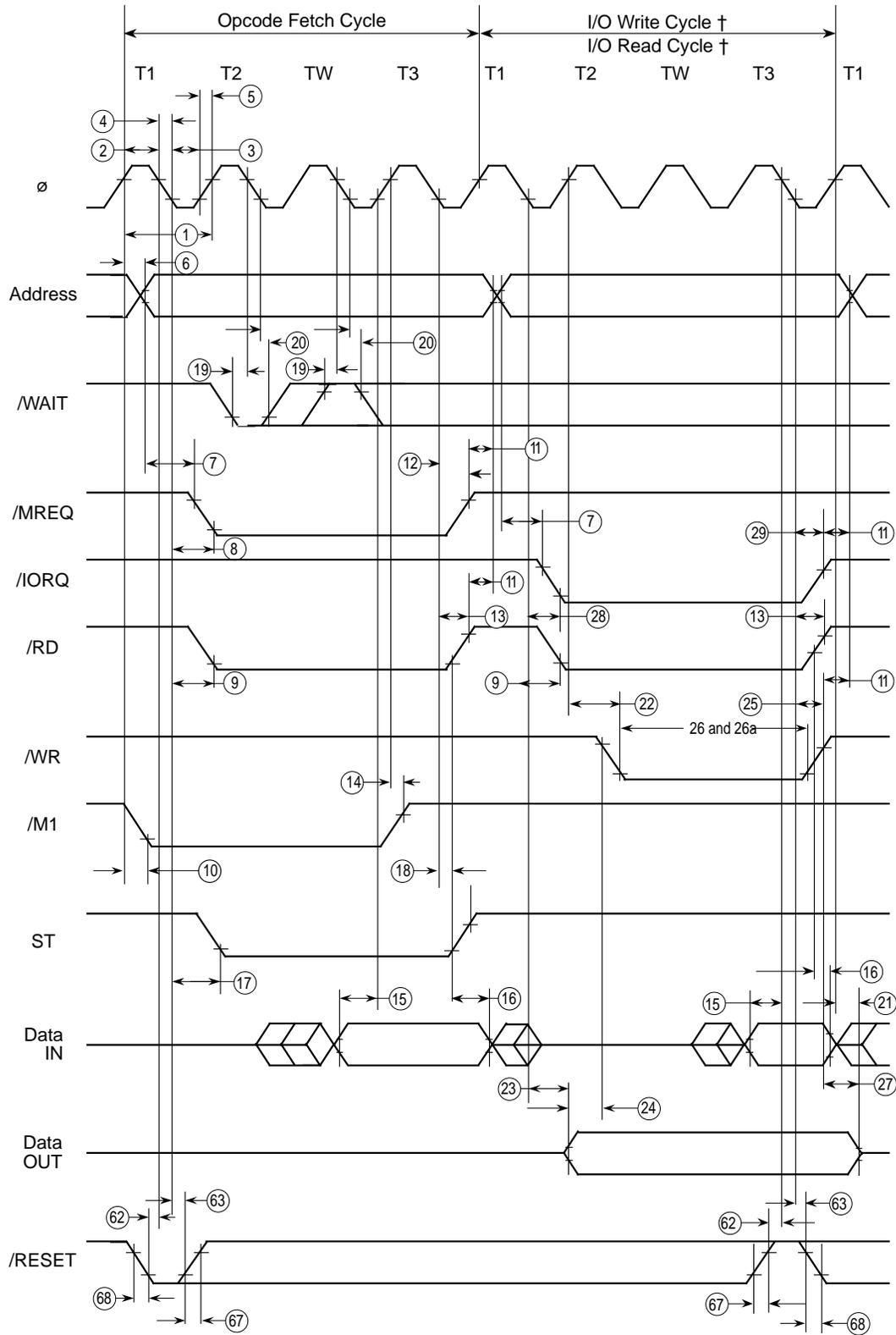
**Figure 90. CPU Timing**
