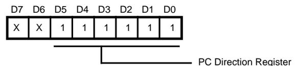
**Figure 87. PC, Port C, Data Direction Register**
