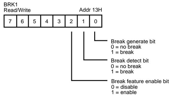
Figure 20. ASCII Break Control Register (Ch. 1)
