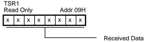
Figure 18. ASCII Receive Data Register (Ch. 1)
