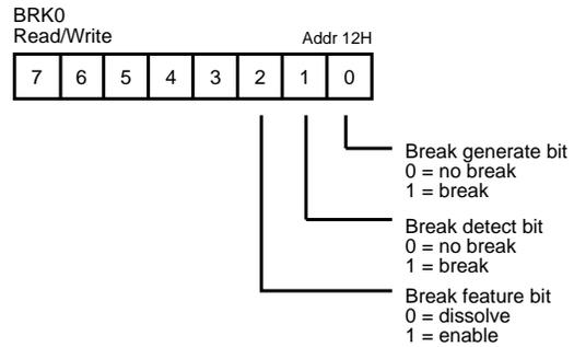
Figure 19. ASCII Break Control Register (Ch. 0)
