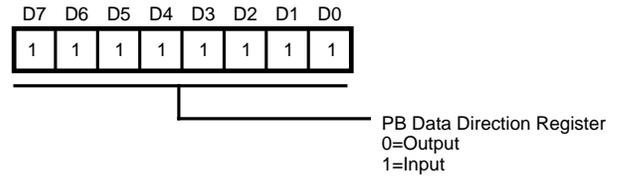
**Figure 85. PB, Port B, Data Direction Register**
