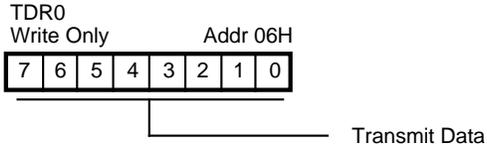
Figure 15. ASCII Transmit Data Register (Ch. 0)
