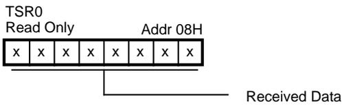
Figure 17. ASCII Receive Data Register (Ch. 0)
