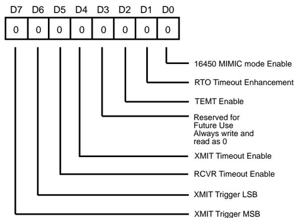
**Figure 64. FIFO Status and Control Register**
