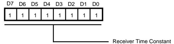
**Figure 68. Receive Time Constant Register**
