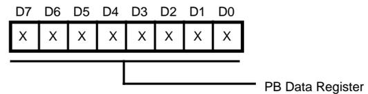
**Figure 86. PB, Port B, Data Register**
