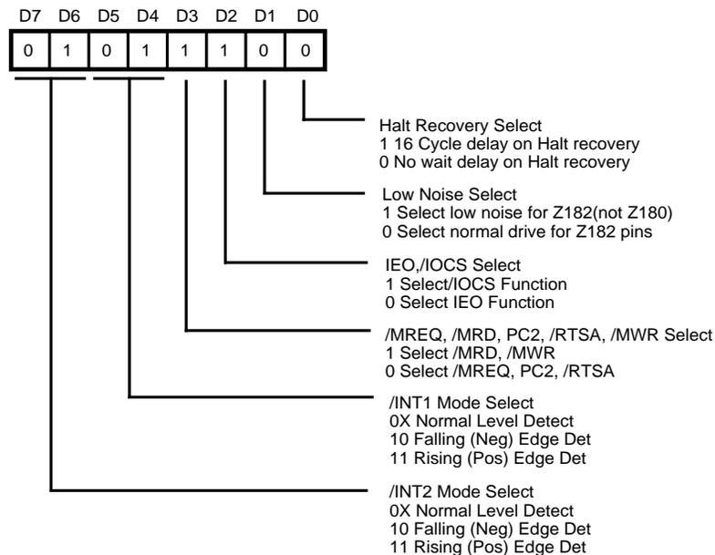
**Figure 59. Interrupt Edge/Pin MUX Register**
