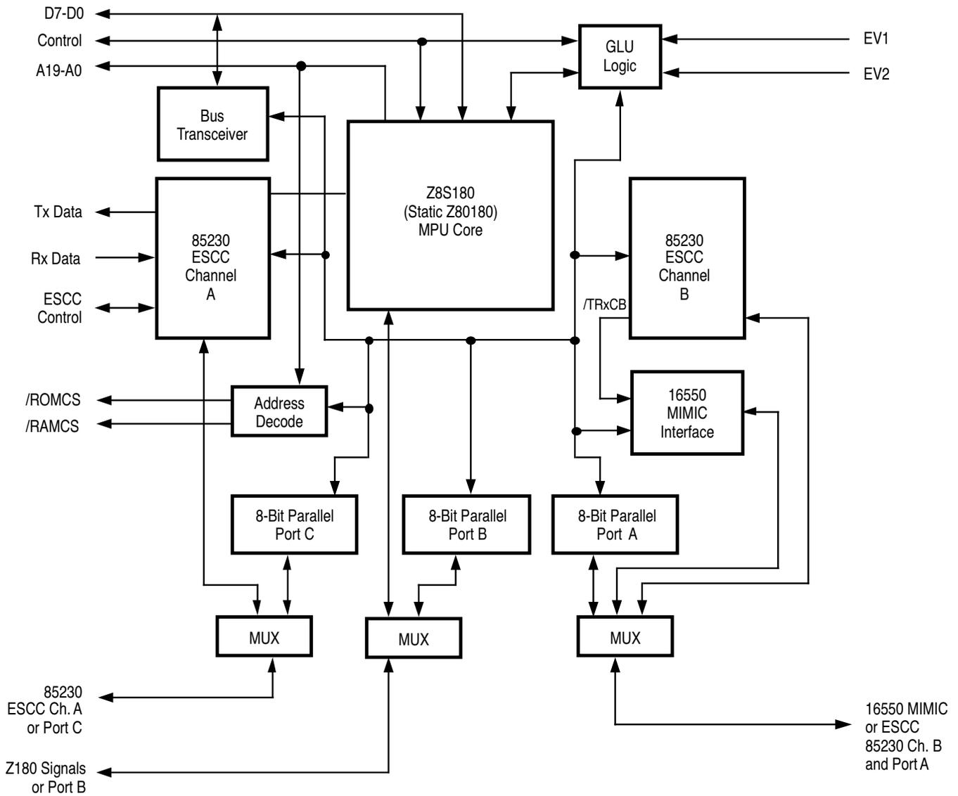
**Note:** Conventional use of the term "MPU side" refers to all interface through the Z180 MPU core and "PC side" refers to all interface through the 16550 MIMIC interface.
