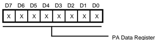
**Figure 84. PA, Port A, Data Register**
