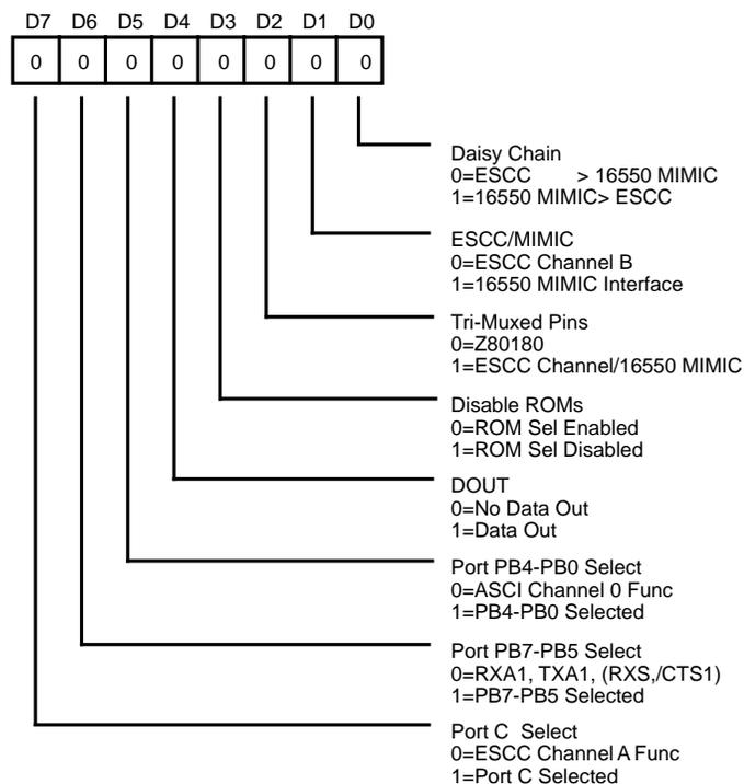
**Figure 54. System Configuration Register**
