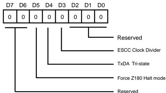
**Figure 82. Z80182 Enhancements Register**
