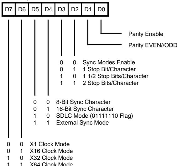
Figure 52. Write Register Bit Functions
