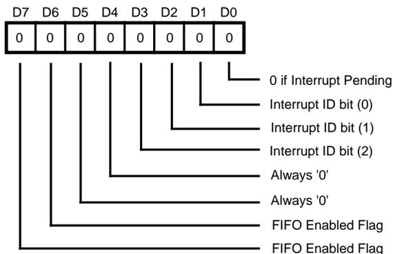
**Figure 73. Interrupt Identification Register**
