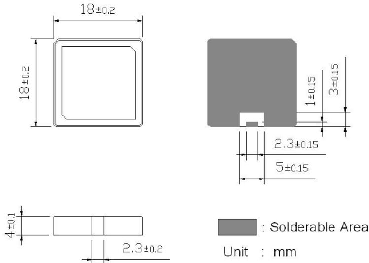
Fig. 1 Mechanical Data
