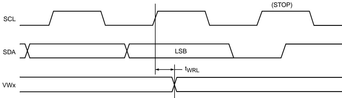
Write Protect and Device Address Pins Timing
