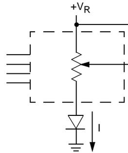
Two terminal Variable Resistor;
