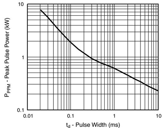
Fig. 2 - Peak Pulse Power Rating Curve
