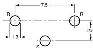
R = rotor, S = stator
