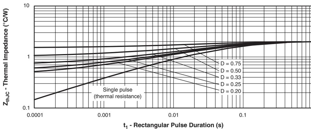
Fig. 4 - Maximum Thermal Impedance  $Z_{thJC}$  Characteristics
