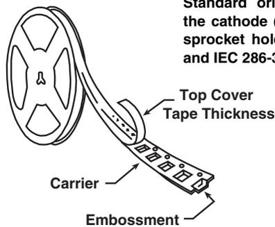
Standard orientation is with the cathode (-) nearest to the sprocket holes per EIA-481-1 and IEC 286-3.
