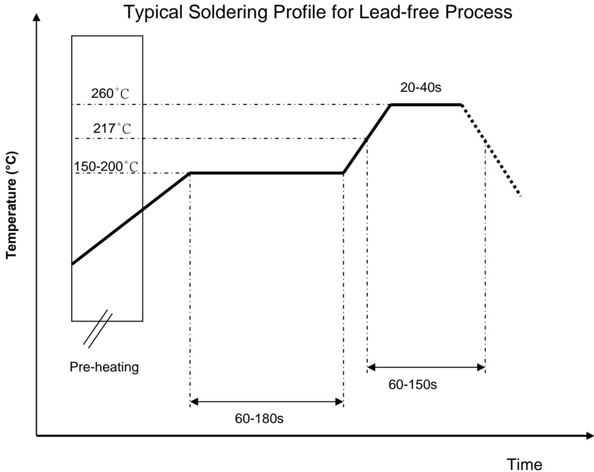
\*Recommended solder paste alloy: SAC305 (Sn96.5 /Ag3 /Cu0.5) Lead Free solder paste
