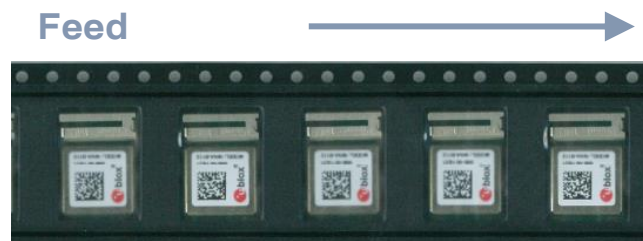
Figure 13: Orientation of NINA-B112 modules on tape
