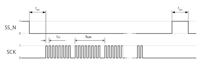
Figure 3: SPI timing diagram
