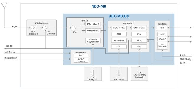
Figure 1: NEO-M8 block diagram
