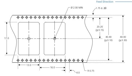
Figure 5: Dimensions and orientation for NEO-M8 modules on tape
