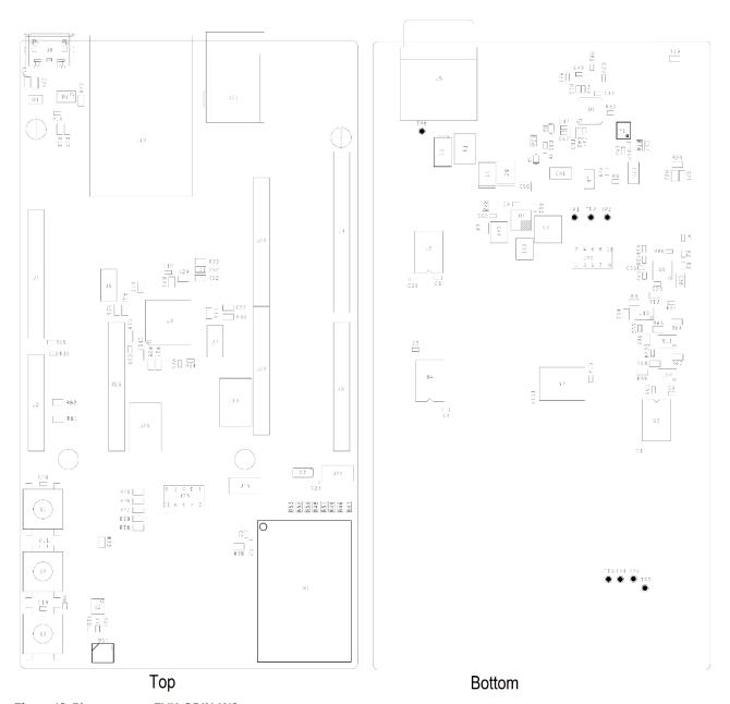
Figure 10: Placement on EVK-ODIN-W2
