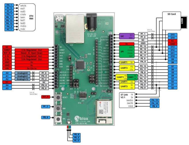
Figure 2: EVK-ODIN-W2 connectors and pin assignment
