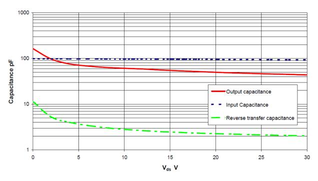
Figure 5 - Typical CV Characteristics.
