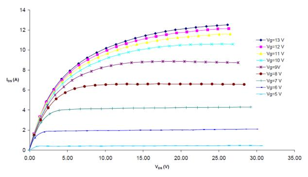
Figure 4 – Typical IV Characteristics.
