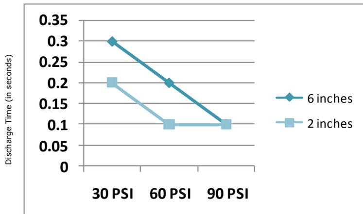
Offset voltage and discharge time per ANSI/ESD STM3.1 using a charged plate monitor with a 20pF, 6" x 6" plate. 1000 to 100 volts. Typical results.
