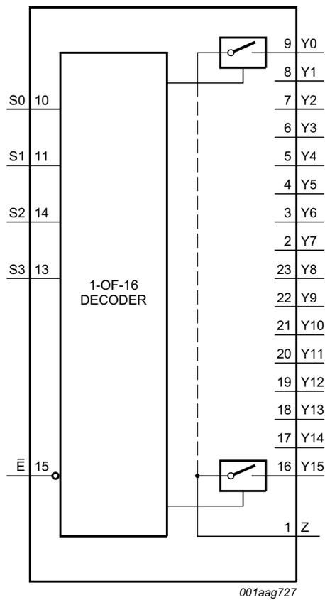
Fig 4. Functional diagram
