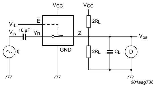
**Fig 15. Test circuit for measuring total harmonic distortion**
