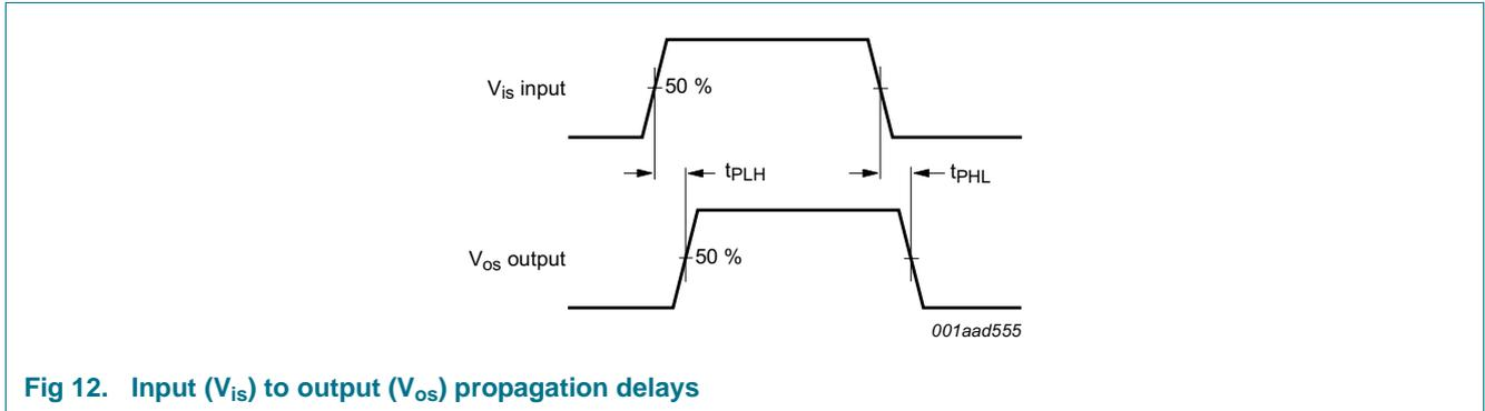
Fig 12. Input ( $V_{is}$ ) to output ( $V_{os}$ ) propagation delays
