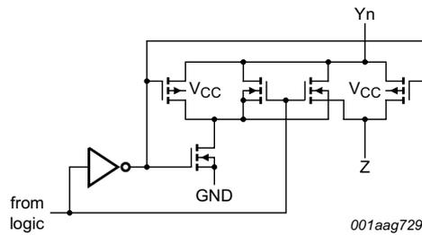
Fig 3. Schematic diagram (one switch)
