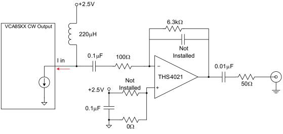
Figure 1. CW Output Circuit
