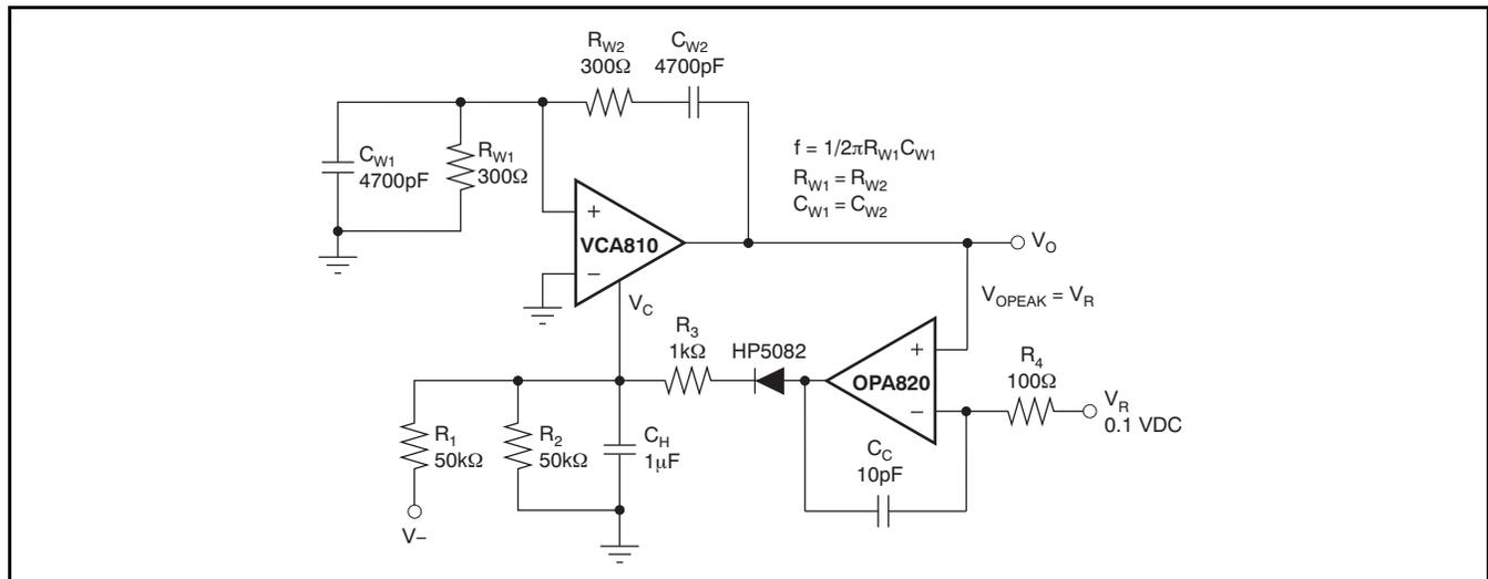
Figure 34. Amplitude-Stabilized Oscillator
