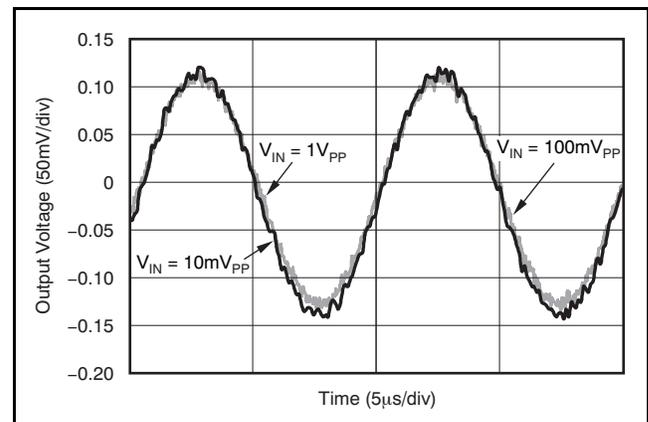
**Figure 33. AGC Output Voltage for 100kHz Sinewave at 10mV<sub>PP</sub>, 100mV<sub>PP</sub>, and 1V<sub>PP</sub>**
