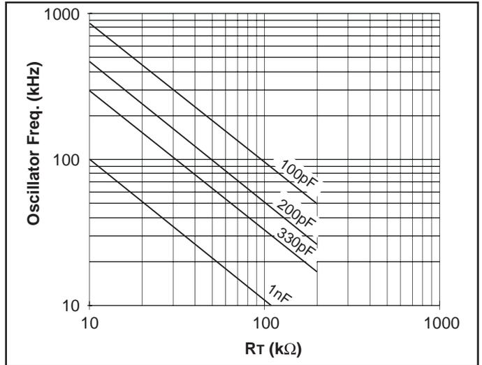
Figure 6. UCC3813-3/-5 oscillator frequency vs.  $R_T$  and  $C_T$ .
