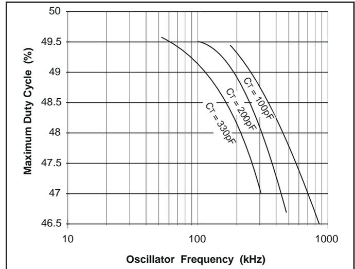
Figure 7. UCC3813-1/-4/-5 max. duty cycle vs. oscillator frequency.
