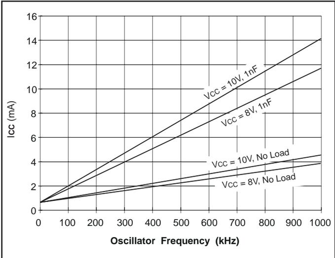
Figure 8. UCC3813-0 I<sub>CC</sub> vs. oscillator frequency.
