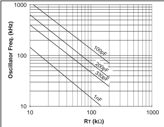
Figure 3. UCC3813-0/-1/-2/-4 oscillator frequency vs.  $R_T$  and  $C_T$ .
