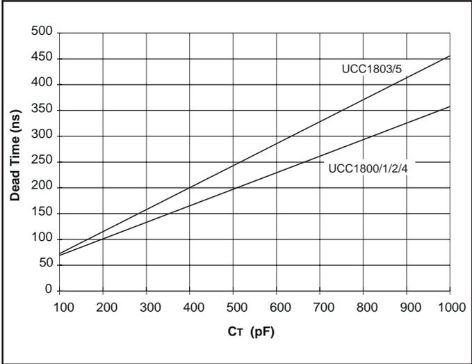
Figure 9. Dead time vs. C<sub>T</sub>, R<sub>T</sub> = 100k.
