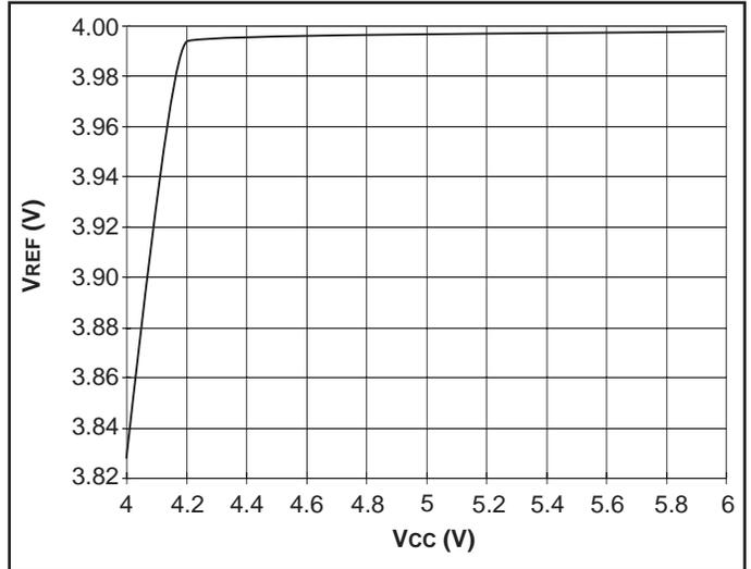
Figure 5. UCC3813-3/-5  $V_{REF}$  vs.  $V_{CC}$ ;  $I_{LOAD} = 0.5mA$ .
