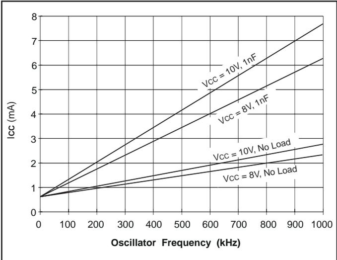
Figure 10. UCC3813-5 I<sub>CC</sub> vs. oscillator frequency.
