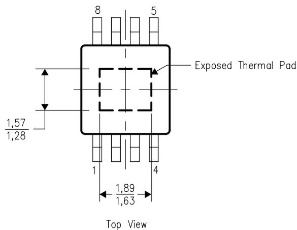
NOTE: All linear dimensions are in millimeters
