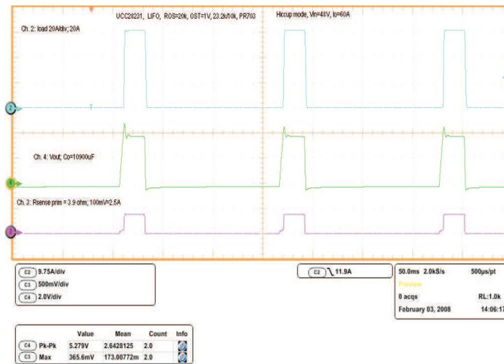
Figure 43. Hiccup Mode with Cycle-by-Cycle Current Limit at  $I_{OUT} = 60$  A
