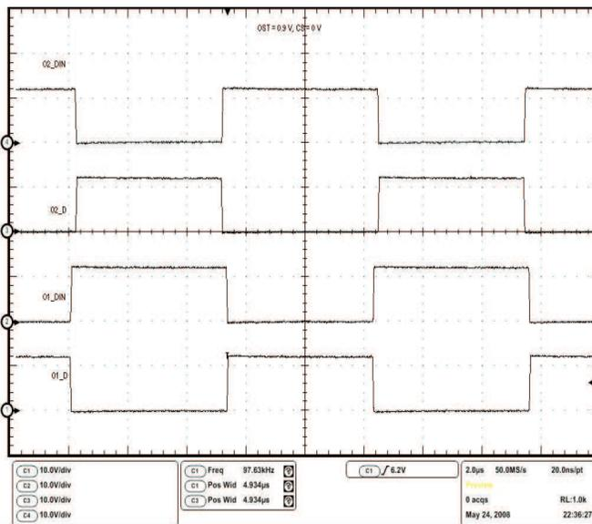
Figure 26. O1\_D and O2\_D Duty cycle Matching at V<sub>CS</sub> = 0.0 V and V<sub>OST</sub> = 1 V
