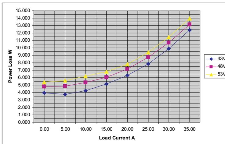
Figure 56. . Power Dissipation
