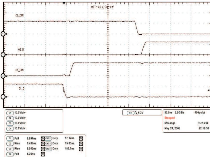
Figure 30. Output Waveforms During Second Half Switching Cycle at  $V_{CS} = 0 V$  and  $V_{OST} = 1 V$
