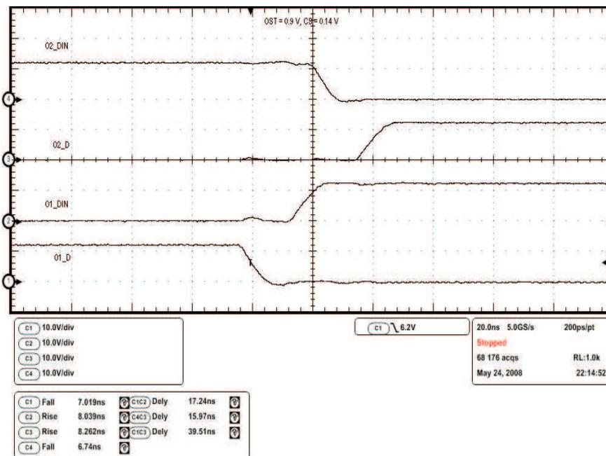
Figure 28. Output Waveforms During Second Half Switching Cycle at  $V_{CS} = 0.14\text{ V}$  and  $V_{OST} = 1\text{ V}$
