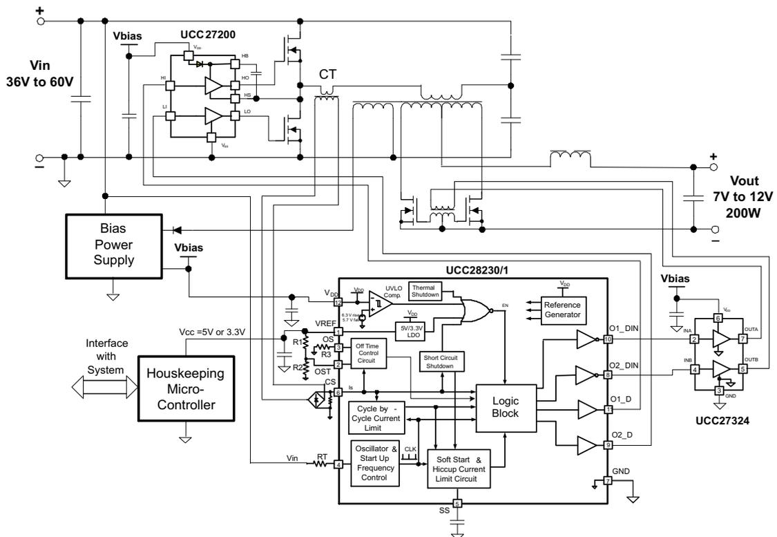
Figure 2. Half-Bridge Bus Converter with Control-Driven Synchronous Rectifier
