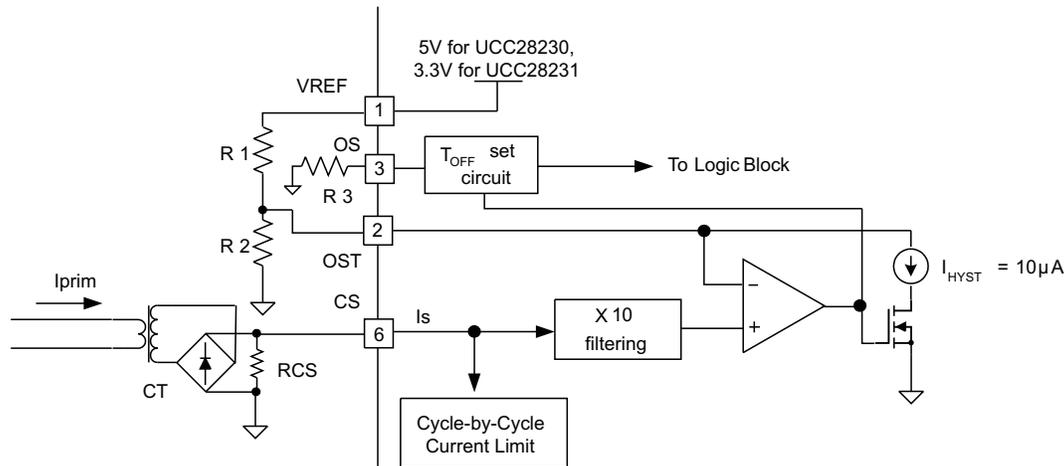
Figure 50. The Off-Time Control Circuit Using Comparator With Hysteresis
