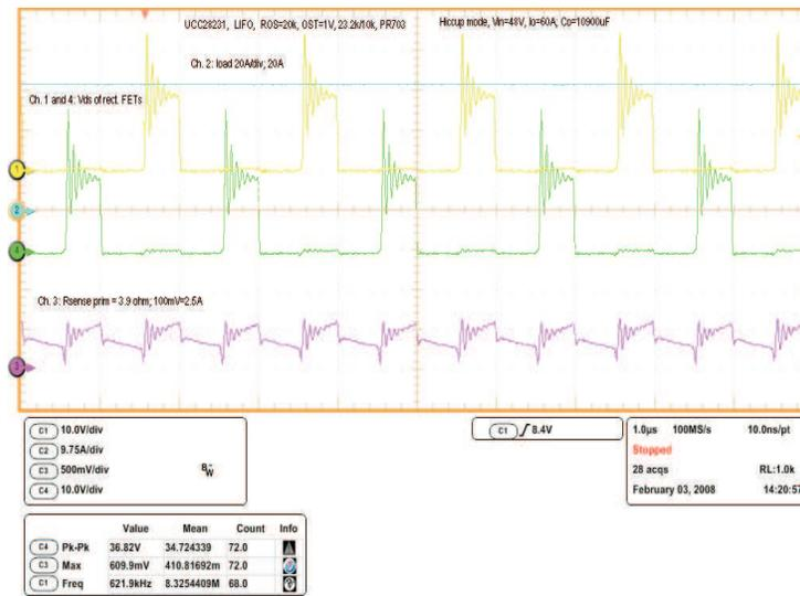
Figure 42. Cycle-by-Cycle Current Limit
