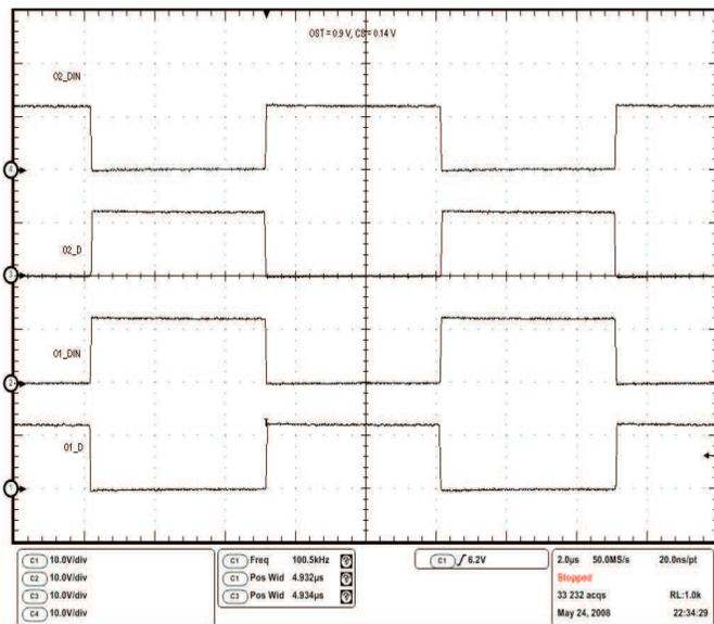
Figure 25. O1\_D and O2\_D Duty Cycle Matching at V<sub>CS</sub> = 0.14 V and V<sub>OST</sub> = 1 V
