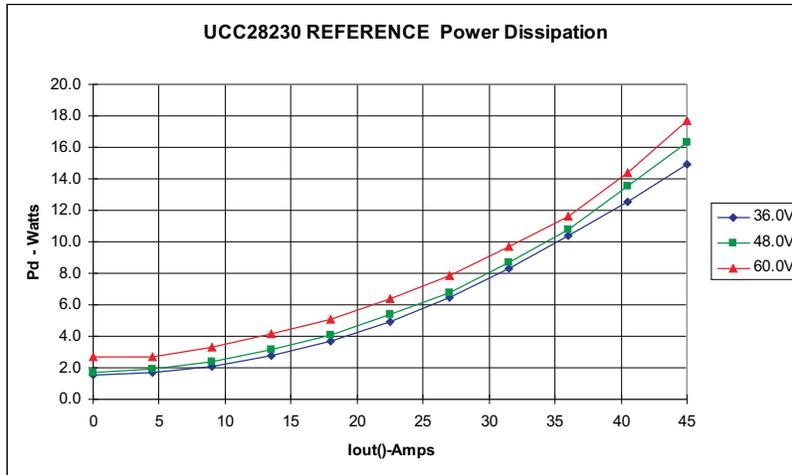
Figure 60. Power Dissipation
