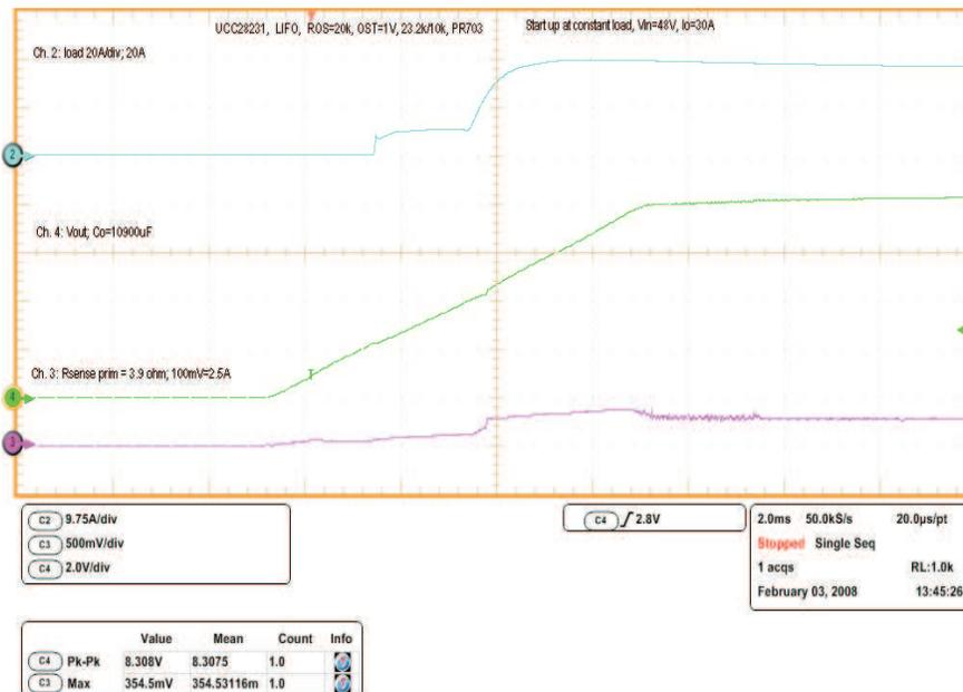
Figure 40. Start up at 30-A Constant Current Load With  $C_O = 10900 \mu\text{F}$
