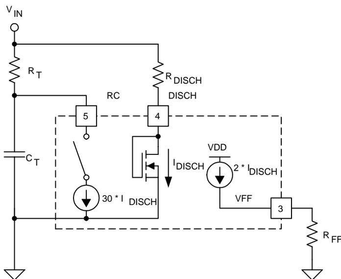
Figure 2. Duty Cycle Clamp (MODE = 1)
