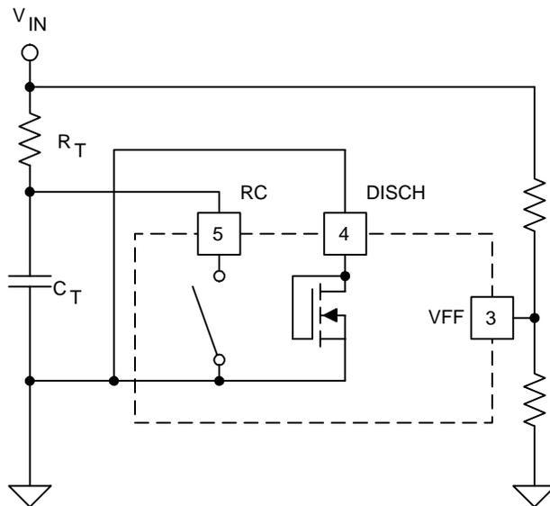
Figure 3. Oscillator Without Clamp (MODE = 0)
