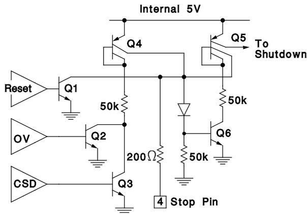
The Error Latch consists of Q5 and Q6 which, when both on, turns off the PWM Output and pulls the Slow-Start pin low. This latch is set by either the Over-Voltage or Current Shutdown comparators, or by a high signal on Pin 4. Reset is accomplished by either the Reset comparator or a low signal on Pin 4. An activation time delay can be provided with an external capacitor on Pin 4 in conjunction with the  $\approx 100\mu\text{A}$  collector current from Q4.
