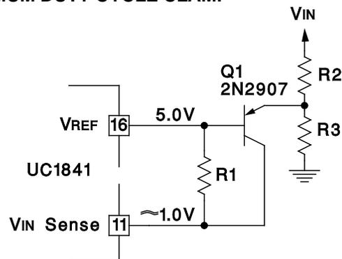
In this circuit,  $R_1$  is used in conjunction with  $C_R$  (not shown) to establish a minimum ramp charging current such that the ramp voltage reaches 4.2V at the required maximum output pulse width.
