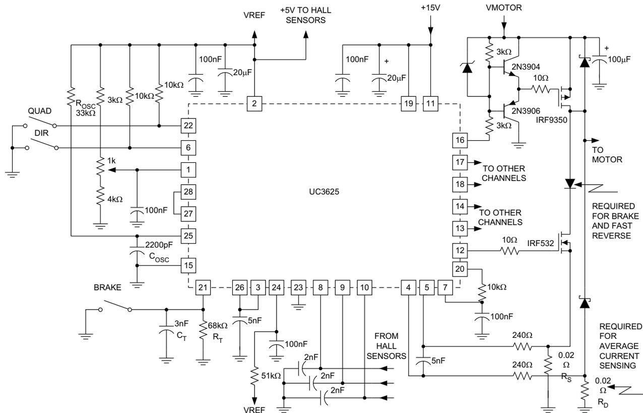
**Figure 14. 45-V/8-A Brushless DC Motor Drive Circuit**
