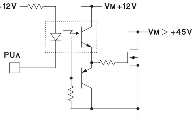
Figure 10. Optocoupled N-Channel High-Side Driver
