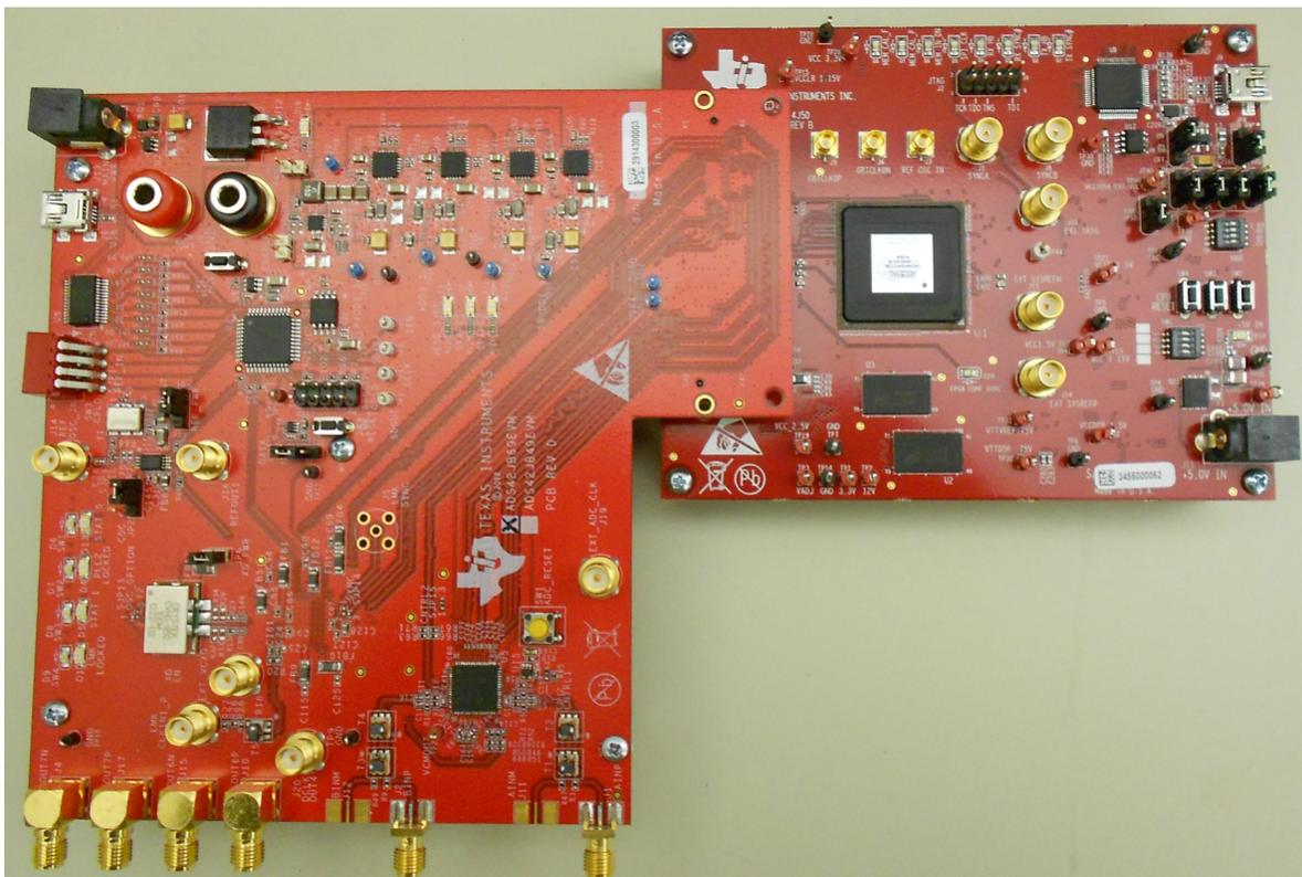
**Figure 64. TSW14J50 EVM Connected to an ADS42JB69 EVM**
