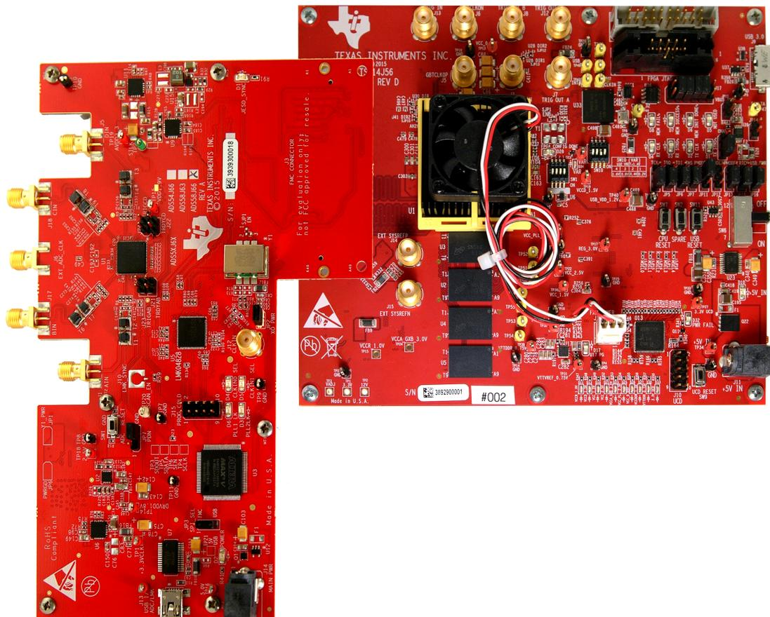
Figure 60. TSW14J56 EVM connected to an ADS58J63 EVM
