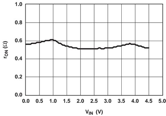
Figure 3.  $r_{on}$  vs  $V_{COM}$  ( $V_+ = 5\text{ V}$ )
