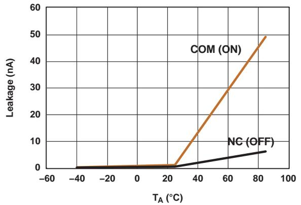
Figure 4. Leakage Current vs Temperature ( $V_+ = 5\text{ V}$ )
