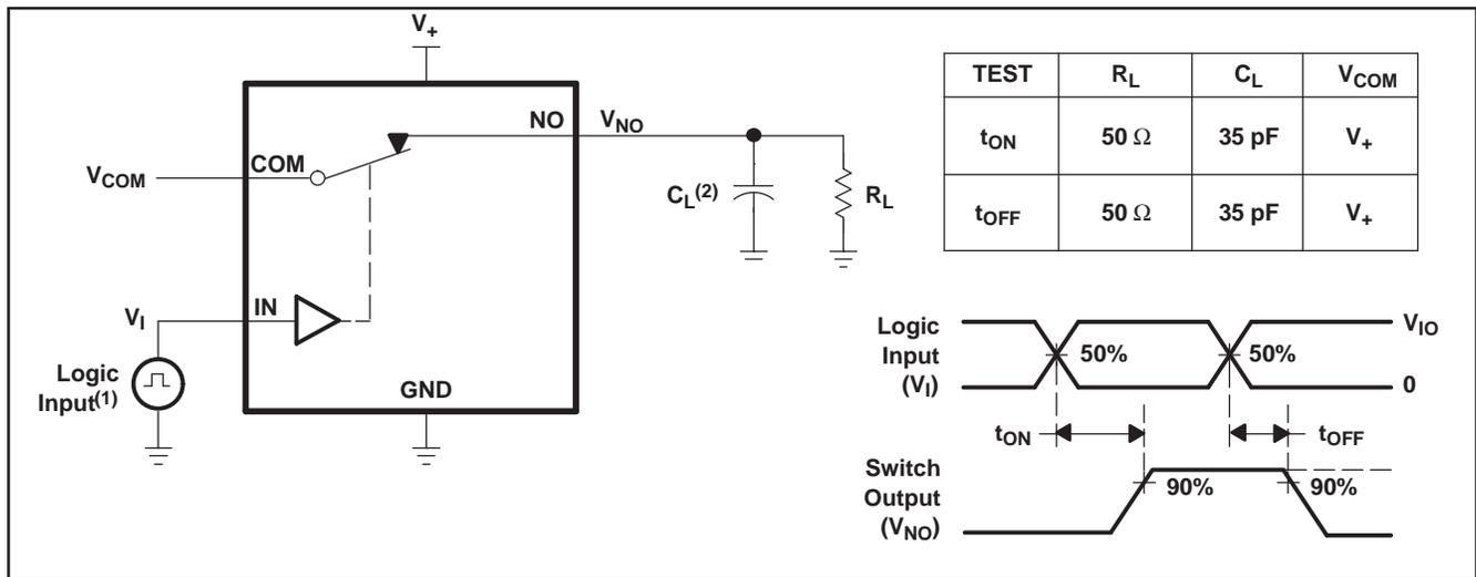
(1) All input pulses are supplied by generators having the following characteristics: PRR  $\leq$  10 MHz,  $Z_O = 50 \Omega$ ,  $t_r < 5$  ns,  $t_f < 5$  ns.
