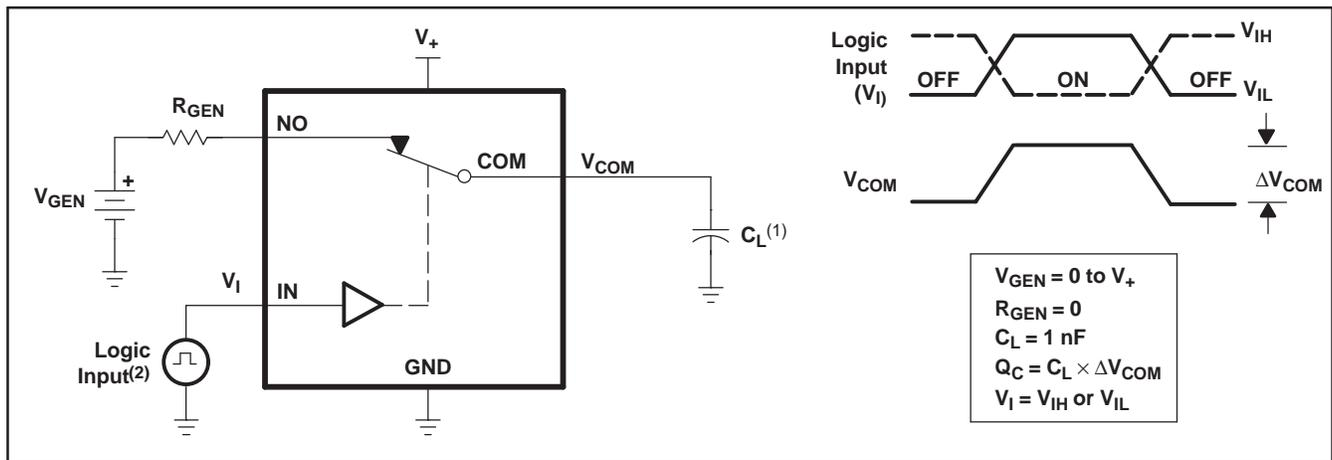
(1)  $C_L$  includes probe and jig capacitance.
