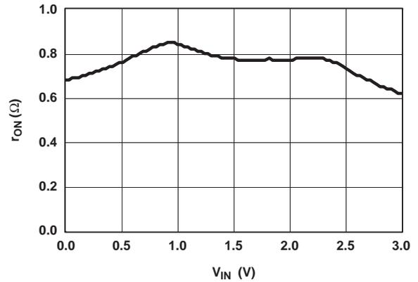
Figure 2.  $r_{on}$  vs  $V_{COM}$  ( $V_+ = 3.3\text{ V}$ )
