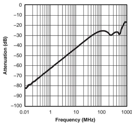
Figure 11. OFF Isolation vs Frequency (V<sub>+</sub> = 5 V)
