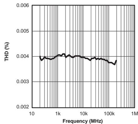
Figure 12. Total Harmonic Distortion vs Frequency (V<sub>+</sub> = 2.5 V)
