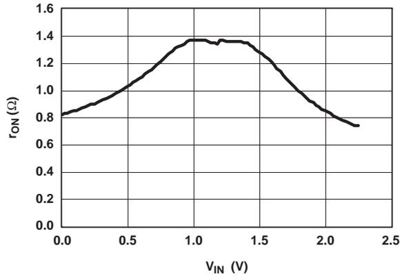
Figure 1.  $r_{on}$  vs  $V_{COM}$  ( $V_+ = 2.5\text{ V}$ )
