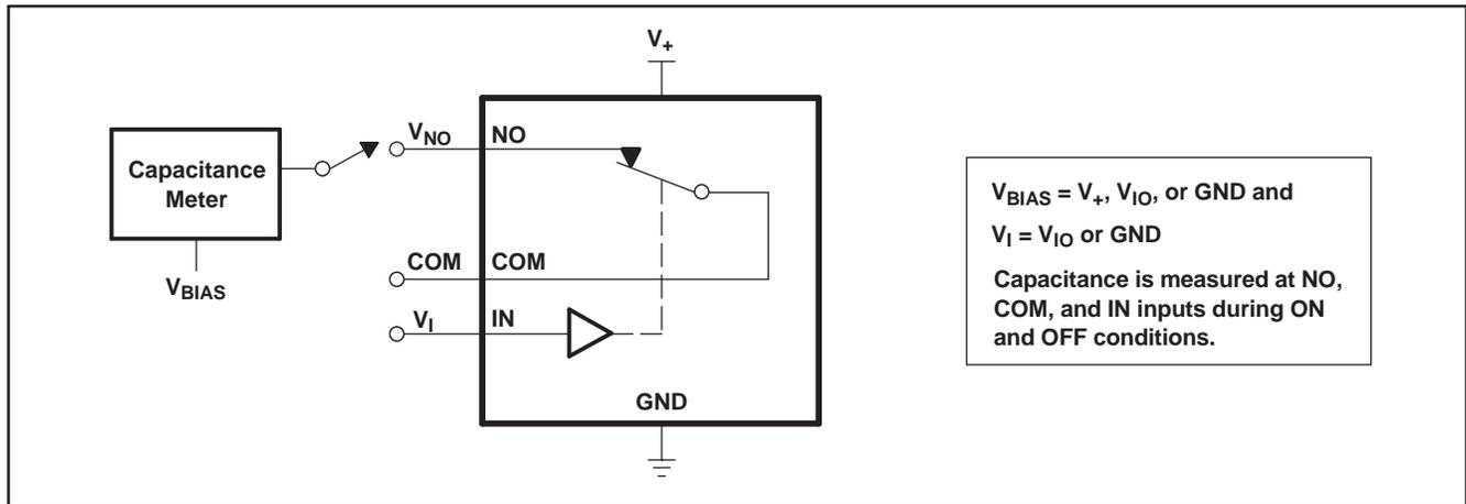
**Figure 17. Capacitance ( $C_I$ ,  $C_{COM(OFF)}$ ,  $C_{COM(ON)}$ ,  $C_{NC(OFF)}$ ,  $C_{NC(ON)}$ )**
