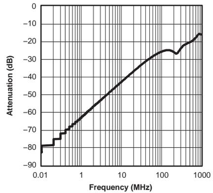
Figure 10. Crosstalk vs Frequency (V<sub>+</sub> = 5 V)
