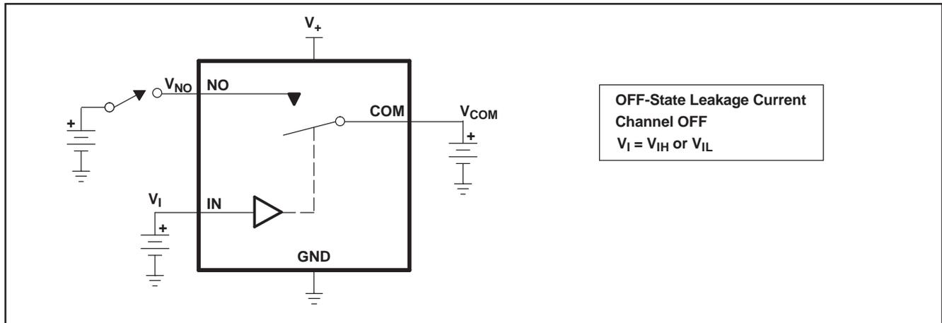
Figure 15. OFF-State Leakage Current ( $I_{COM(OFF)}$ ,  $I_{NC(OFF)}$ ,  $I_{COM(PWROFF)}$ ,  $I_{NC(PWRFF)}$ )
