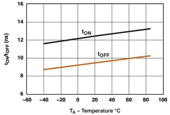
Figure 8. t<sub>ON</sub>/t<sub>OFF</sub> vs Temperature (V<sub>+</sub> = 5 V)
