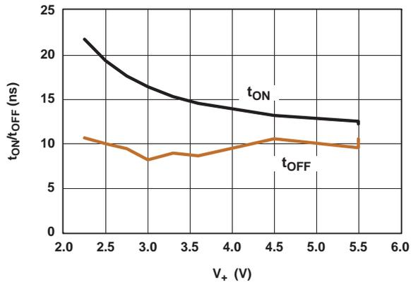
Figure 7. t<sub>ON</sub>/t<sub>OFF</sub> vs Supply Voltage
