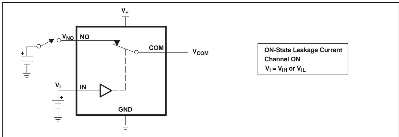
Figure 16. ON-State Leakage Current ( $I_{COM(ON)}$ ,  $I_{NC(ON)}$ )
