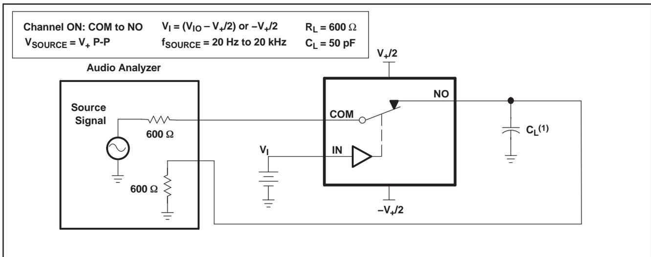
(1)  $C_L$  includes probe and jig capacitance.
