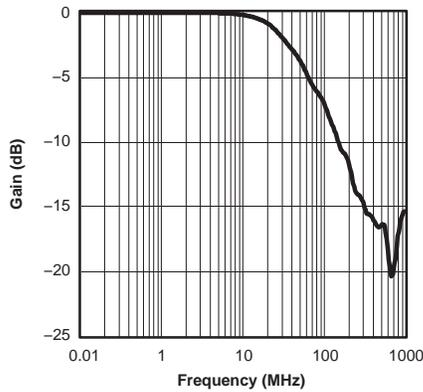
Figure 9. Gain vs Frequency (V<sub>+</sub> = 5 V)
