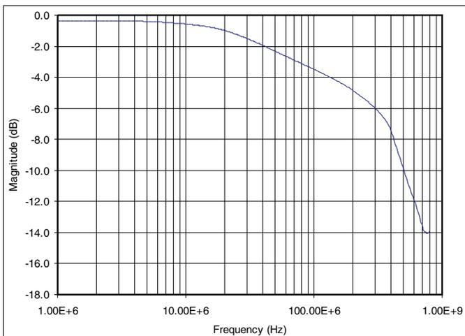
Figure 7. Bandwidth Dual Supply ( $\pm 5$  V)
