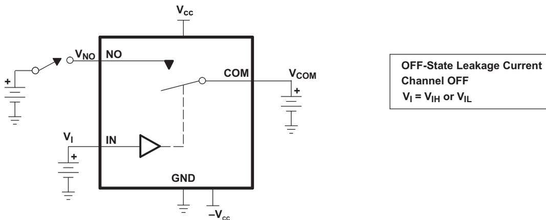
**Figure 13. OFF-State Leakage Current ( $I_{COM(OFF)}$ ,  $I_{NC(OFF)}$ )**
