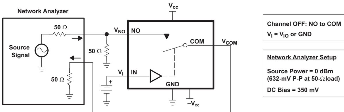
Figure 19. OFF Isolation (O<sub>ISO</sub>)
