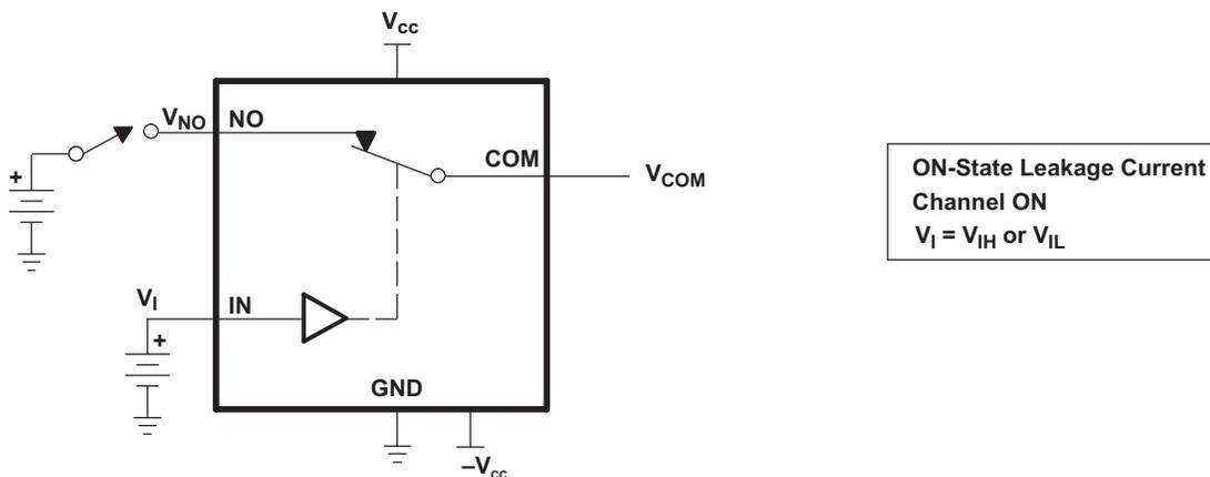
**Figure 14. ON-State Leakage Current ( $I_{COM(ON)}$ ,  $I_{NC(ON)}$ )**
