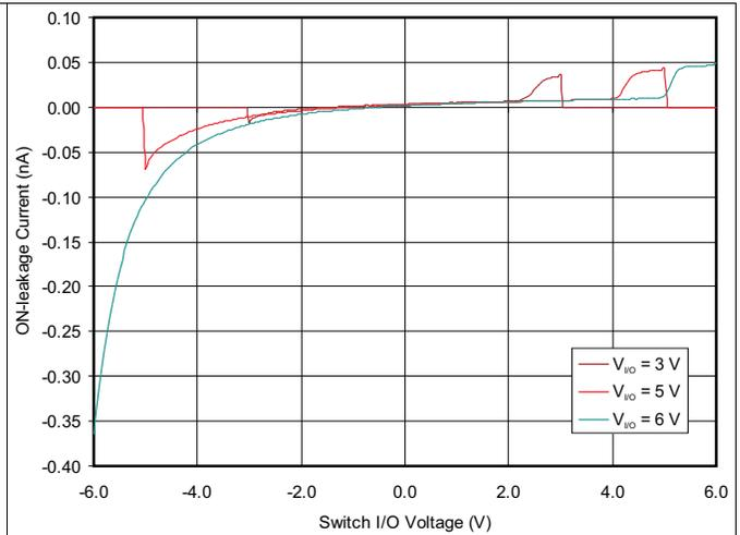
Figure 2. Leakage Current vs I/O voltage (Switch ON)
