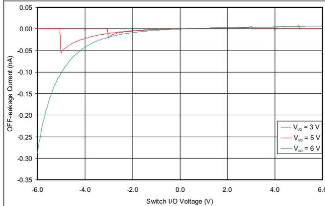
Figure 3. Leakage Current vs I/O Voltage (Switch OFF)
