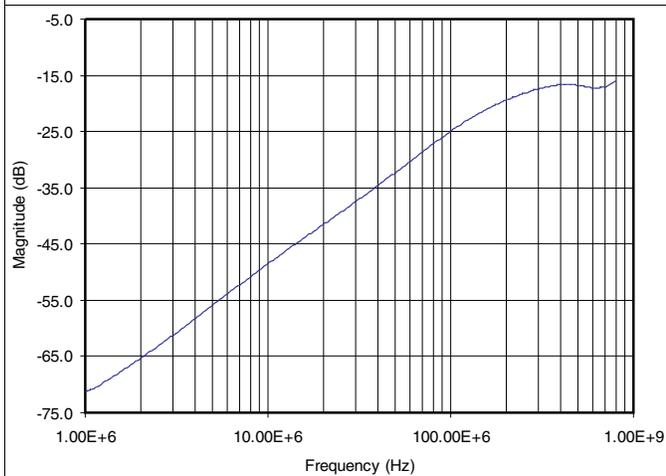
Figure 9. Crosstalk vs Frequency Dual Supply ( $\pm 5$  V)
