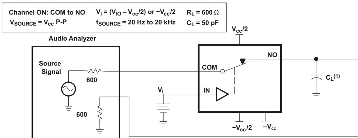
(1)  $C_L$  includes probe and jig capacitance.
