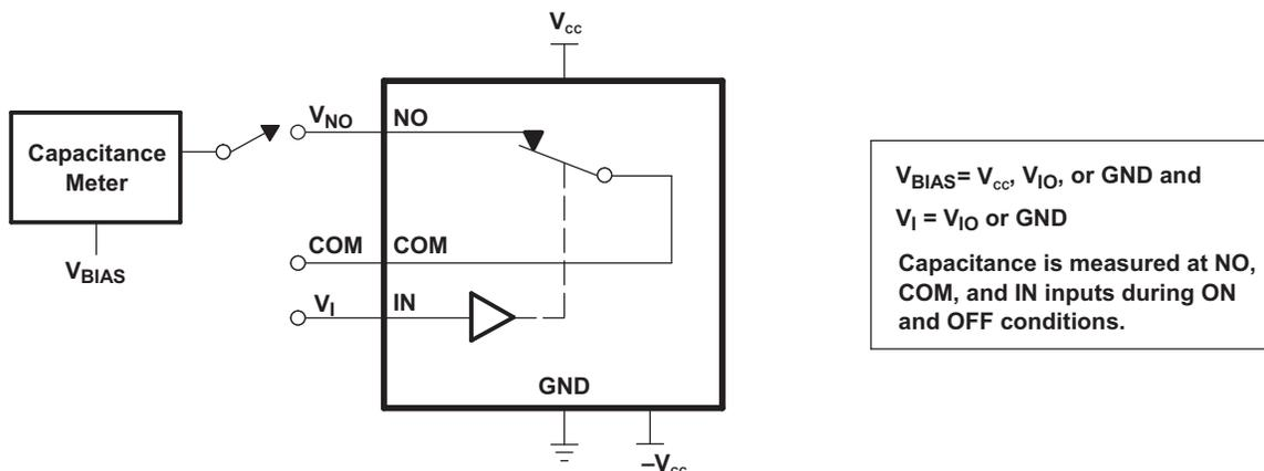
Figure 15. Capacitance ( $C_{COM(OFF)}$ ,  $C_{COM(ON)}$ ,  $C_{NC(OFF)}$ ,  $C_{NC(ON)}$ )
