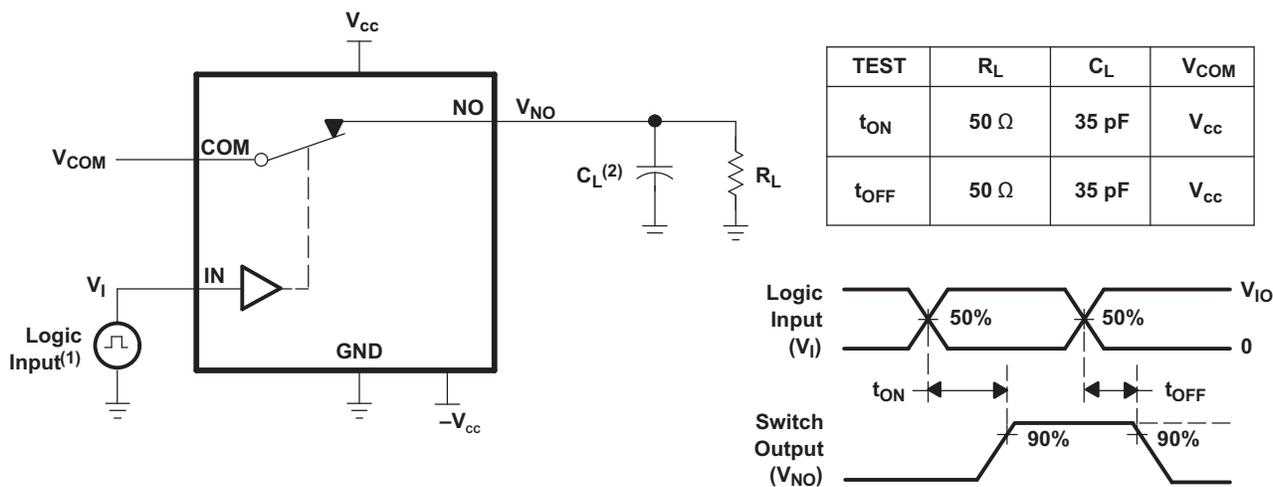
(1) All input pulses are supplied by generators having the following characteristics:  $PRR \leq 10 \text{ MHz}$ ,  $Z_O = 50 \Omega$ ,  $t_r < 5 \text{ ns}$ ,  $t_f < 5 \text{ ns}$ .
