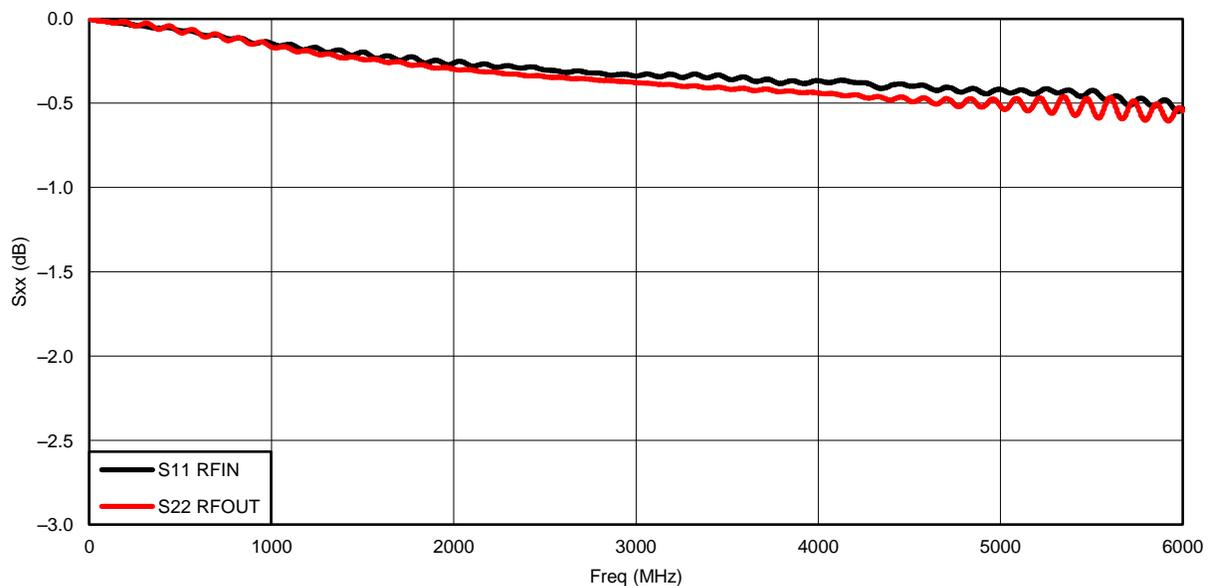
**Figure 6. S11, S22 (Open), U1 and L1 Uninstalled, Copper Tape Replaced C1 and C2**
