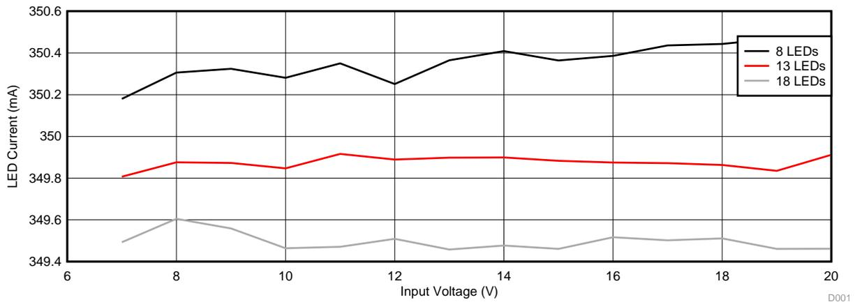
Figure 4. Output LED Current vs Input Voltage
