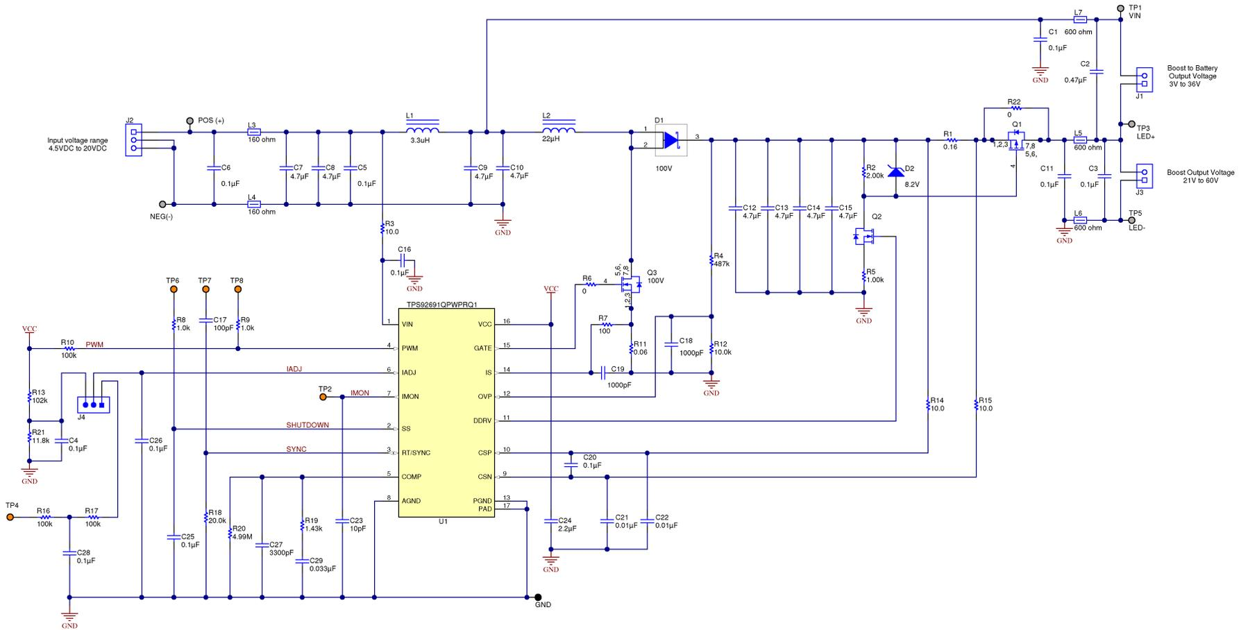
Figure 2. TPS92691EV752 Schematic
