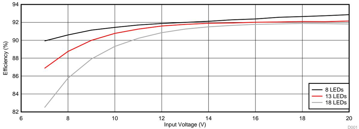
Figure 3. Efficiency vs Input Voltage (350-mA LED Current)
