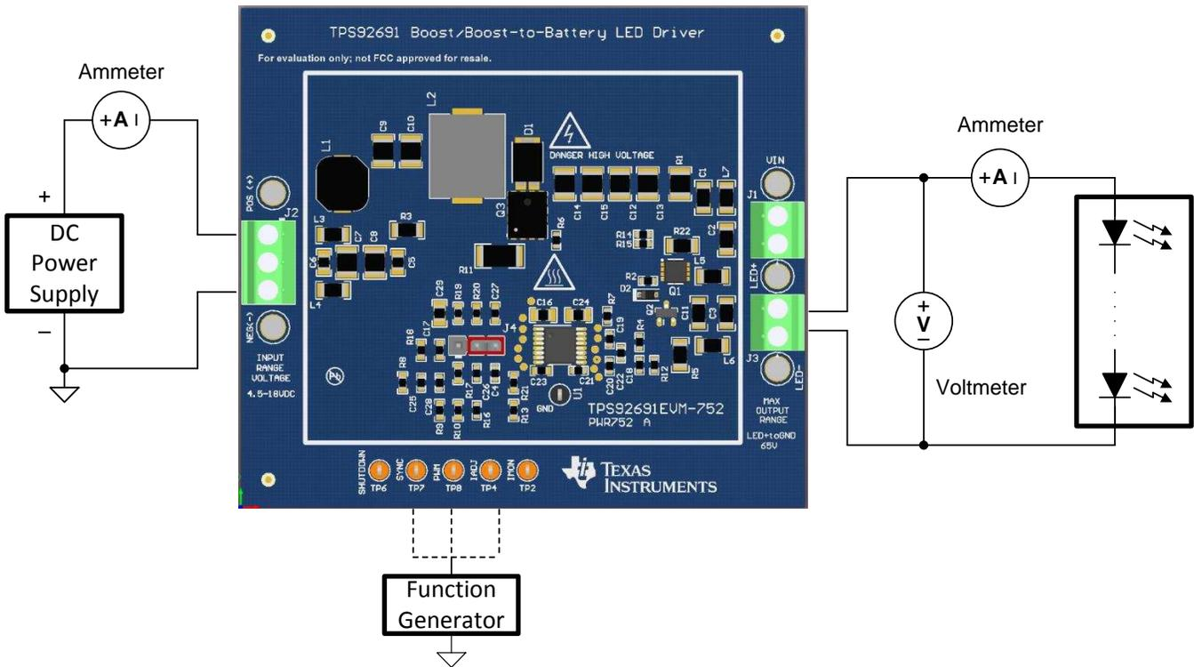
Figure 1. Connection Diagram
