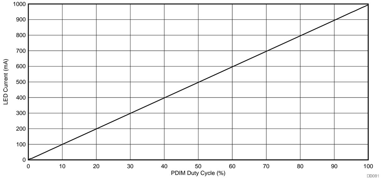
Figure 4. Output Current vs. PWM Duty Cycle (250 Hz)
