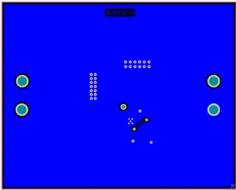
Figure 10. Bottom Layer and Bottom Overlay (Bottom View)
