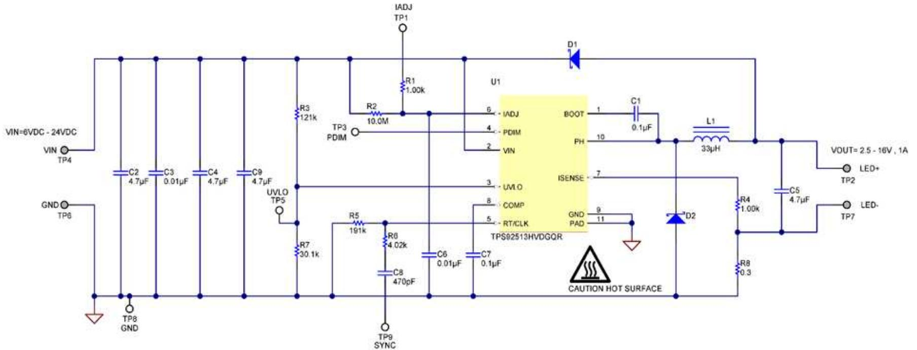
Figure 1. TPS92513EVM-001 Schematic
