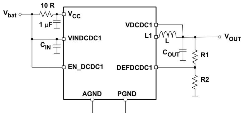
When a resistor divider is connected to DEFDCDC1 or DEFDCDC2, the output voltage can be set from 0.6V up to the input voltage  $V_{bat}$ . The total resistance ( $R1+R2$ ) of the voltage divider should be kept in the 1MΩ range in order to maintain a high efficiency at light load.  $V_{DEFDCDCx} = 0.6V$
