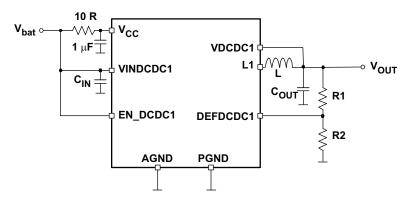
When a resistor divider is connected to DEFDCDC1 or DEFDCDC2, the output voltage can be set from 0.6V up to the input voltage  $V_{bat}$ . The total resistance (R1+R2) of the voltage divider should be kept in the 1M $\Omega$  range in order to maintain a high efficiency at light load.  $V_{DEFDCDCx} = 0.6V$
