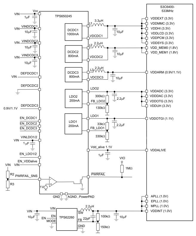
Figure 19. Samsung Processor Configuration
