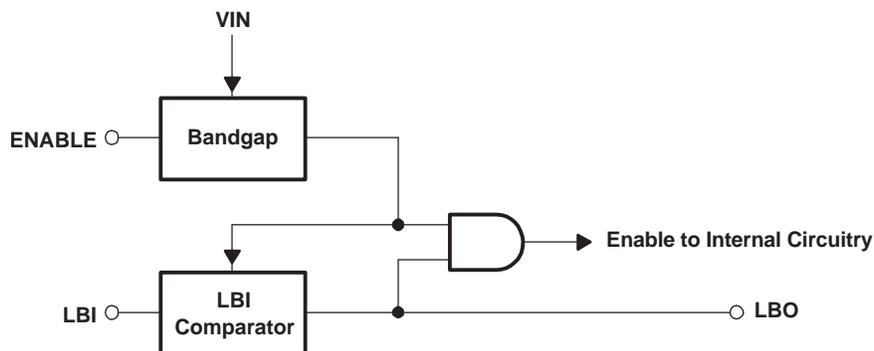
Figure 20. Block Diagram of ENABLE/LBI Functionality for TPS62051
