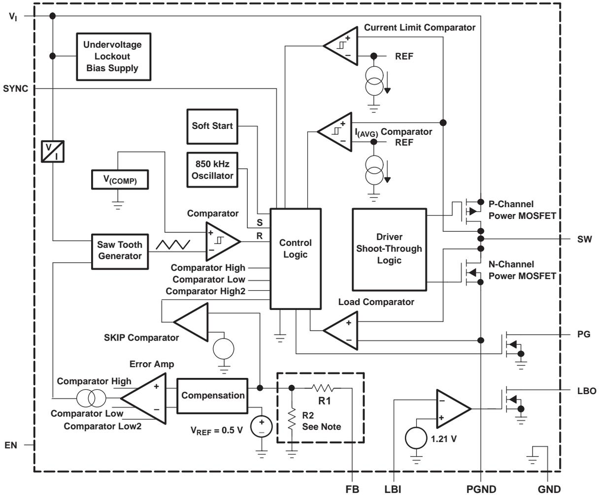
NOTE: For the adjustable versions (TPS62050, TPS62051), the internal feedback driver is disabled and the FB pin is directly connected to the GM amplifier.
