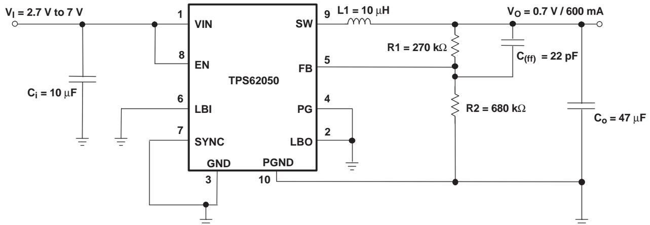
The TPS62050 is used to generate output voltages as low as 0.7 V. With such low output voltages, the inductor discharges very slowly. This leads to a high output voltage ripple in power-save mode (SYNC = GND). It is therefore recommended to use a larger output capacitor to keep the output ripple low. With an output capacitor of 47  $\mu\text{F}$ , the output voltage ripple is less than 40 mV<sub>pp</sub>.
