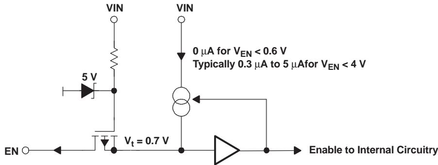
Figure 18. Internal Circuit of the ENABLE Pin
