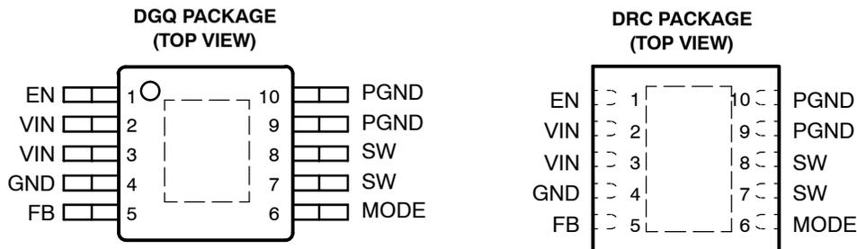
NOTE: The PowerPAD must be connected to GND.
