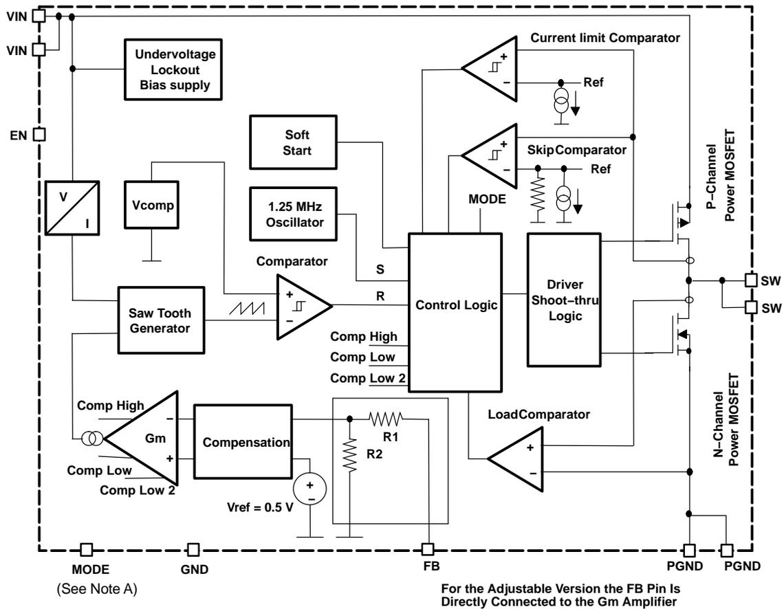
NOTE A: The TPS6202x has an active-high MODE pin. The TPS62021 has an active-low  $\overline{\text{MODE}}$  pin.
