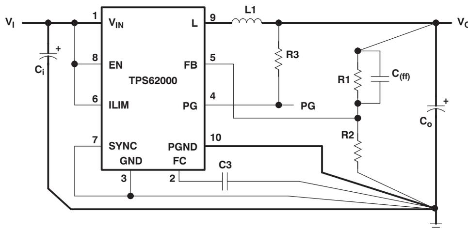
Figure 16. Layout Diagram
