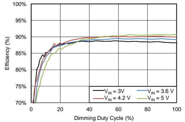
**Figure 6. Efficiency vs Dimming Cycle, 7 LEDs**
