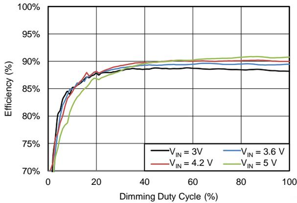
**Figure 5. Efficiency vs Dimming Cycle, 6 LEDs**
