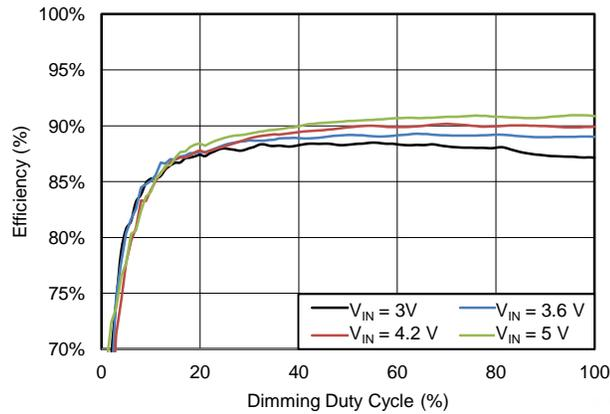
**Figure 7. Efficiency vs Dimming Cycle, 8 LEDs**
