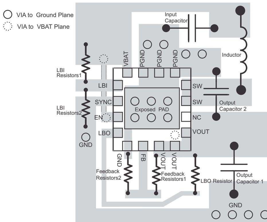
Figure 23. Layout Example Schematic
