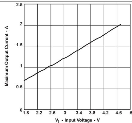
**Figure 2. TPS61092 Maximum Output Current vs Input Voltage**
