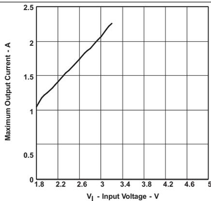
**Figure 1. TPS61091 Maximum Output Current vs Input Voltage**
