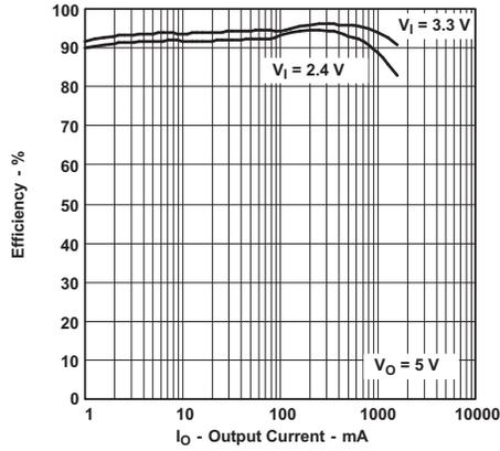
Figure 5. TPS61092 Efficiency vs Output Current
