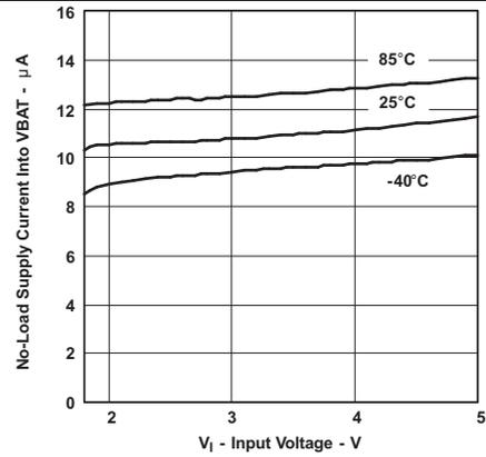
Figure 10. TPS61092 No-Load Supply Current Into VBAT Voltage
