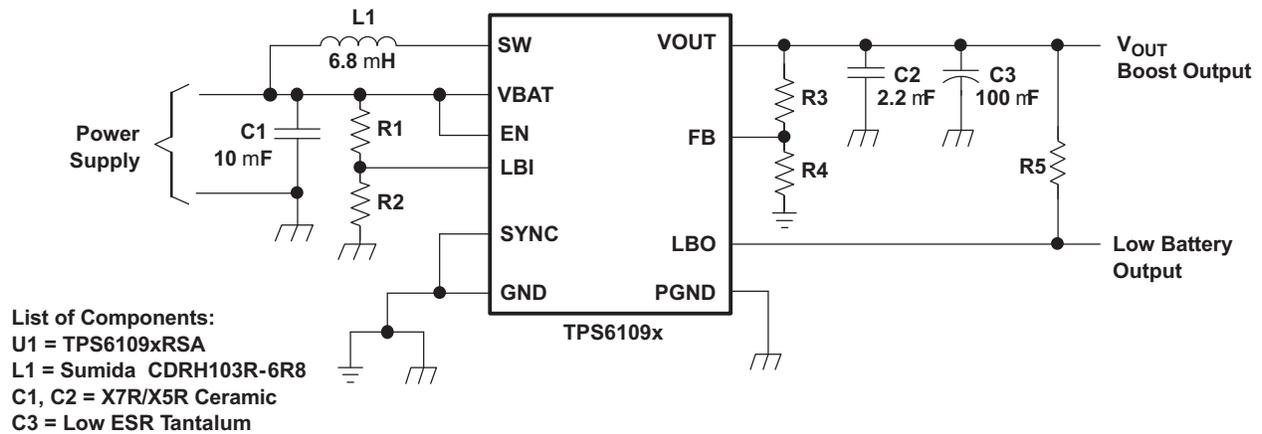
**Figure 13. Parameter Schematic**
