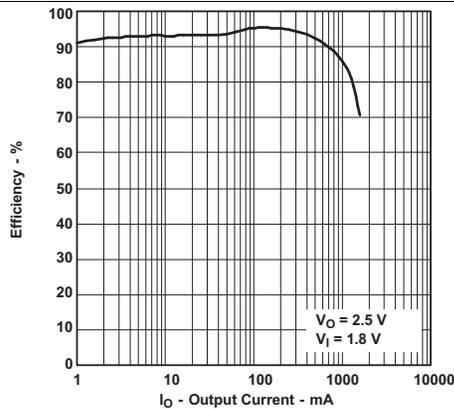
**Figure 3. TPS61090 Efficiency vs Output Current**
