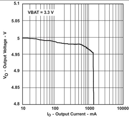
Figure 9. TPS61092 Output Voltage vs Output Current
