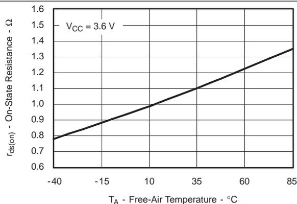
Figure 5.  $r_{ds(on)}$  LED Switch (Q2) vs Temperature
