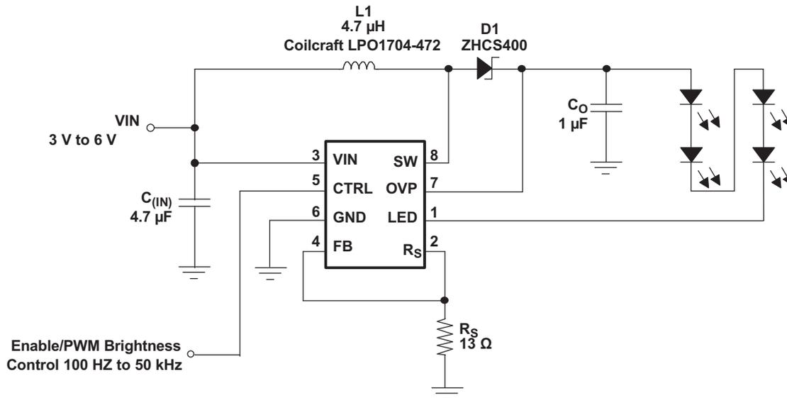
Figure 20. TPS61043 With 1-mm Total System Height
