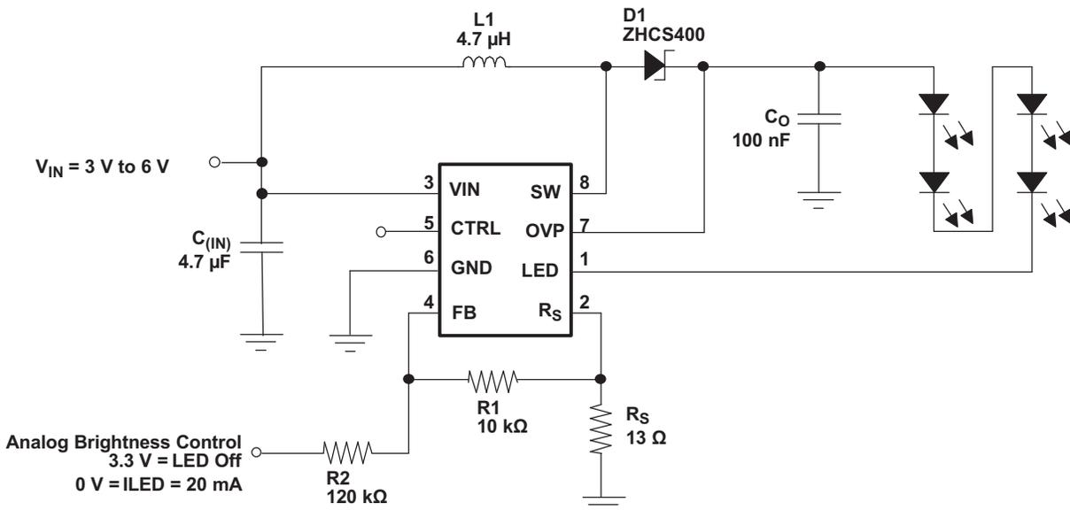
**Figure 23. Adjustable Brightness Control Using an Analog Voltage**
