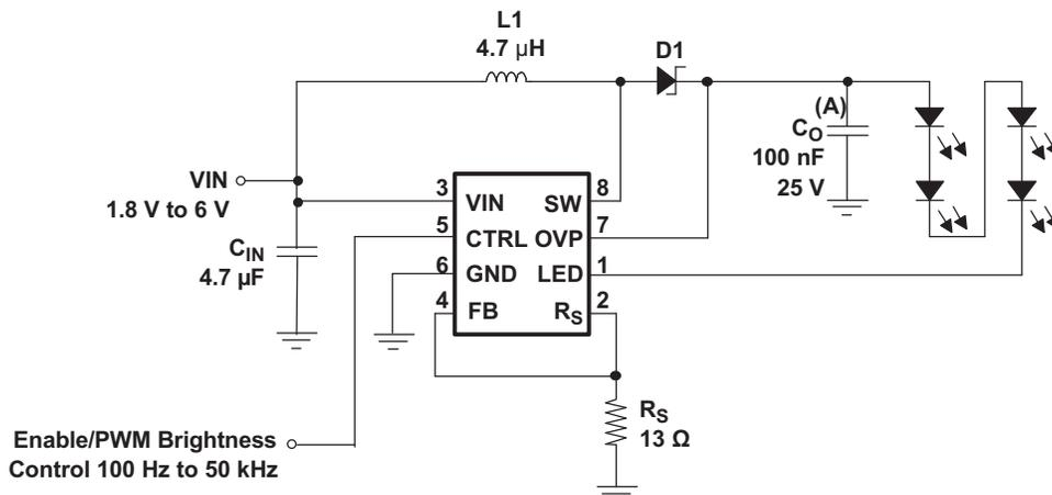
(A) Output capacitor values like 1 μF and larger, reduce the LED ripple current and improve line regulation.
