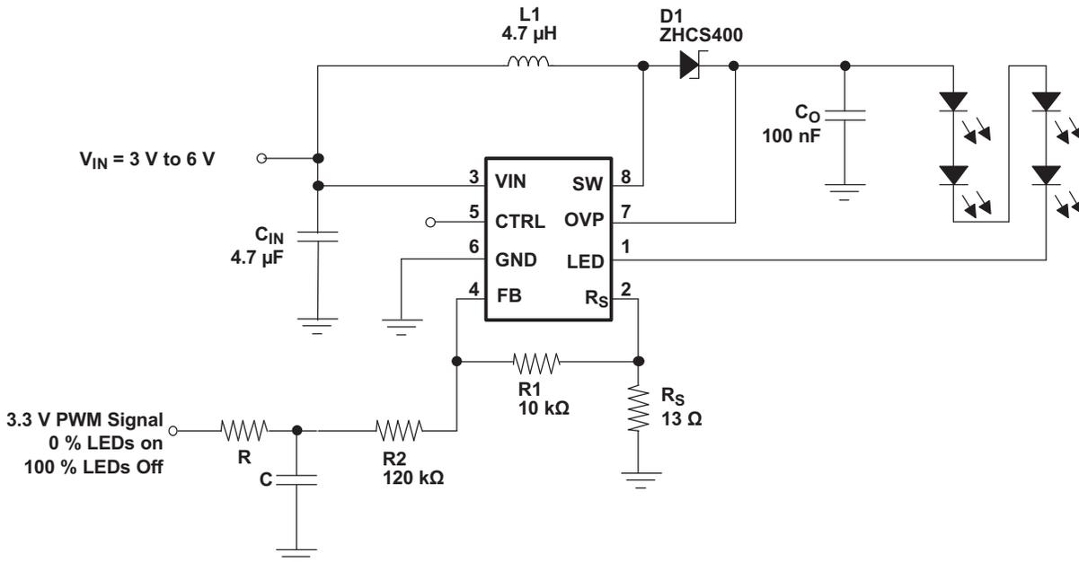
Figure 24. Alternative Adjustable Brightness Control Using PWM Signal
