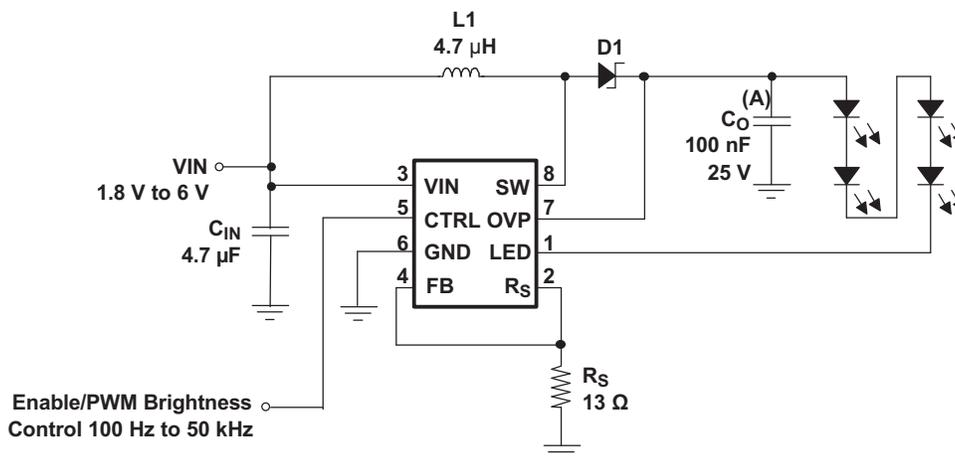
(A) Output capacitor values like 1  $\mu$ F and larger, reduce the LED ripple current and improve line regulation.
