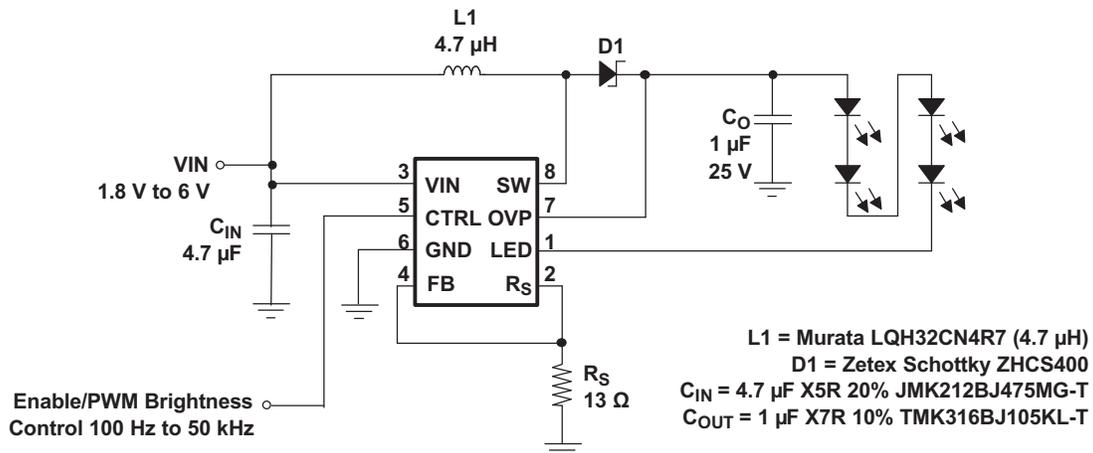
Figure 8. Schematic
