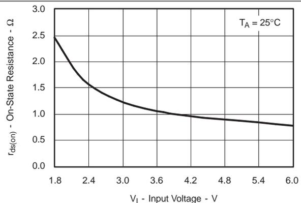
Figure 6.  $r_{ds(on)}$  LED Switch (Q2) vs Input Voltage
