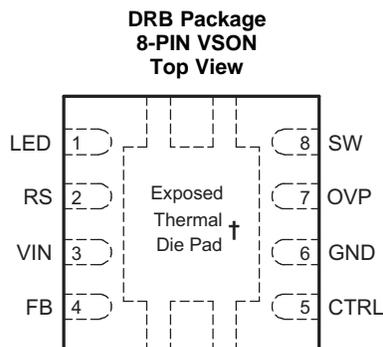
† The exposed thermal die pad is connected to GND.
