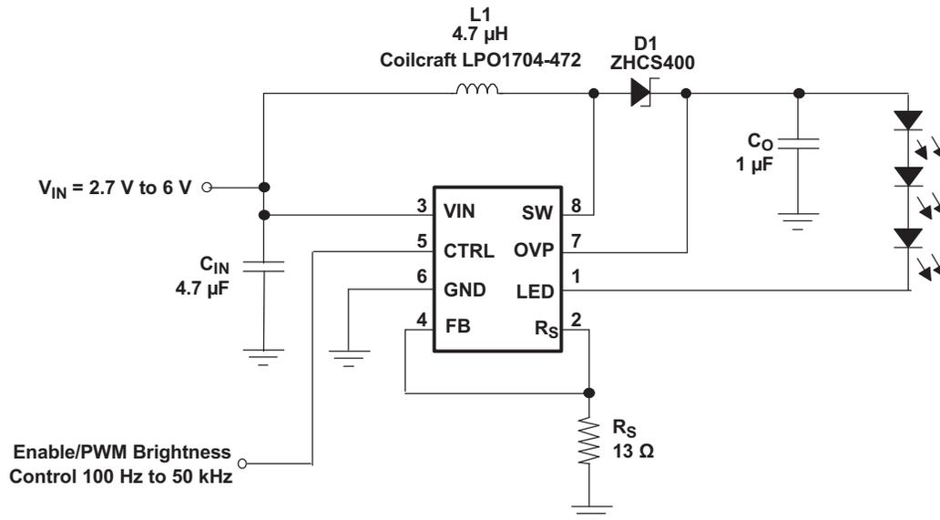
**Figure 22. TPS61043 Powering 3 LEDs**
