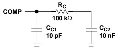
**Figure 23. Compensation of Control Loop**
