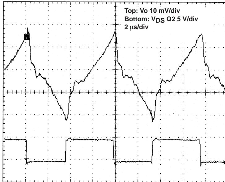
Figure 26. Output Voltage Ripple at 8 A
