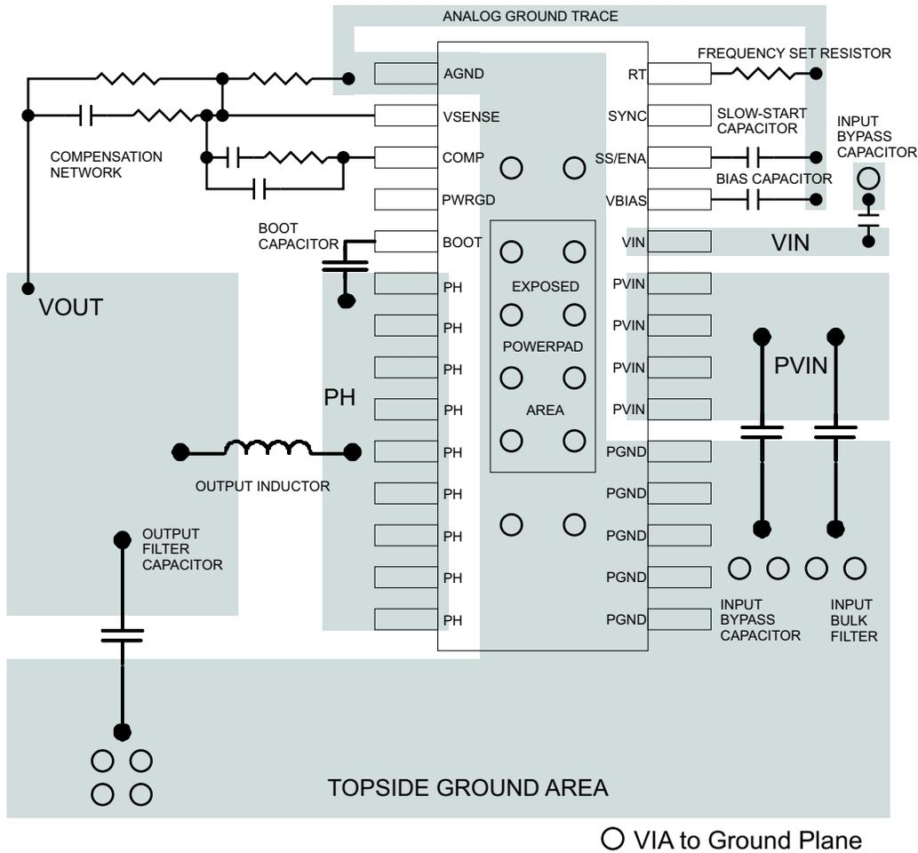
Figure 12. PCB Layout for 28-Pin PWP PowerPAD
