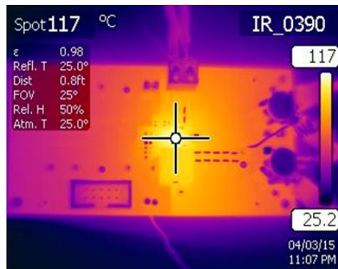
**Figure 17. Thermal Image at 0.95-V Output at 12 V<sub>IN</sub>, 30-A Output**
