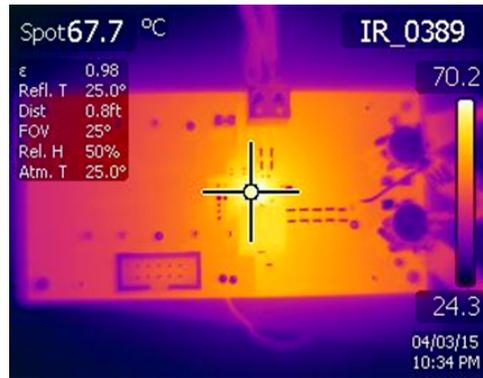
**Figure 16. Thermal Image at 0.95-V Output at 12 V<sub>IN</sub>, 20-A Output**
