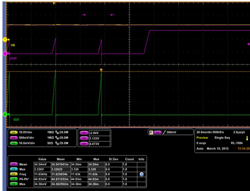
Ch1 =  $V_{IN}$  at 10 V/division, Ch2 =  $I_{IN}$  at 2 A/division, Ch3 =  $V_{OUT}$  at 500 mV/division, Ch4 =  $I_{OUT}$  at 10 A/division
