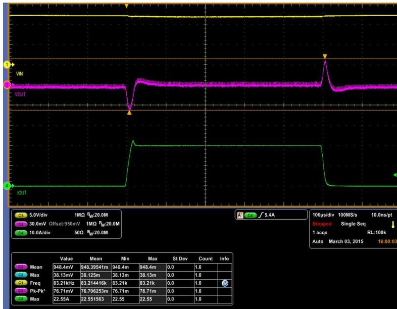
Ch1 =  $V_{IN}$  at 5 V/division, Ch3 =  $V_{OUT}$  at 30 mV/division, Ch4 =  $I_{OUT}$  at 10 A/division
