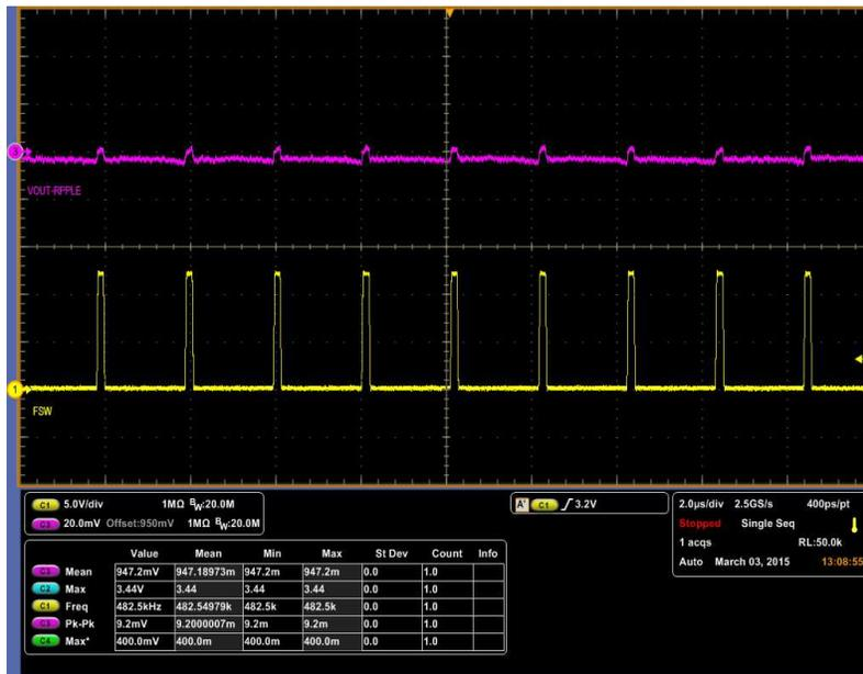
Ch1 = SW at 5 V/division, Ch3 =  $V_{OUT}$  ripple at 20 mV/division
