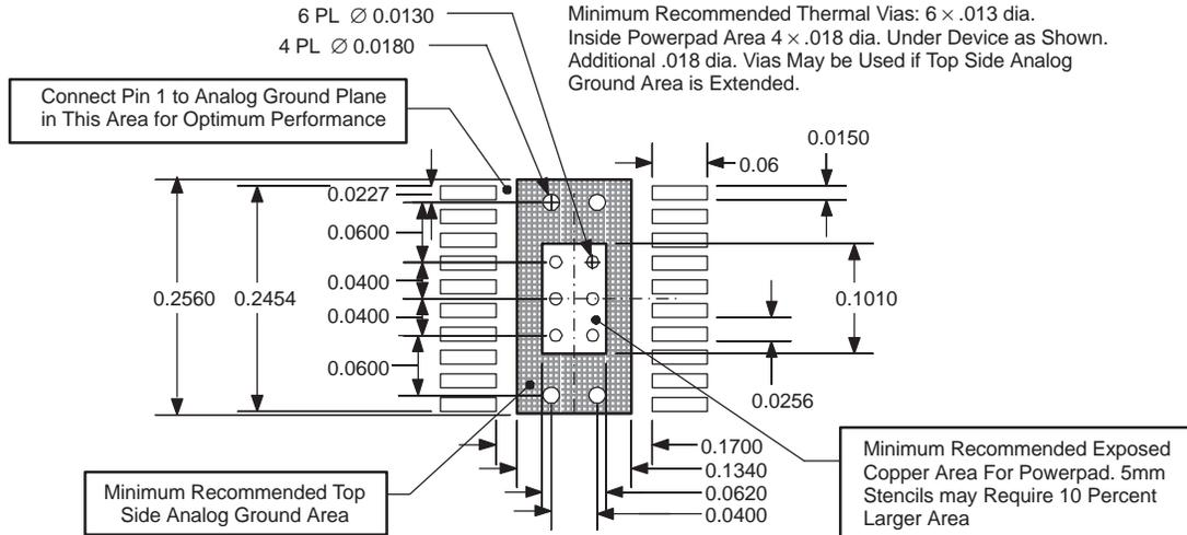
Figure 11. Recommended Land Pattern for 20-Pin PWP PowerPAD
