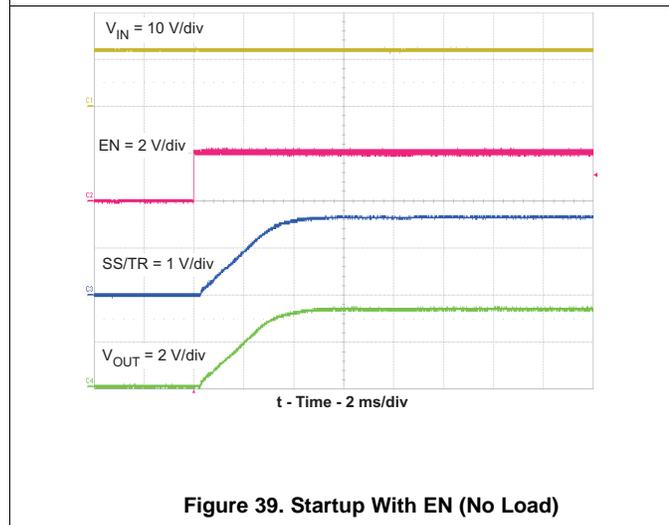
Figure 39. Startup With EN (No Load)
