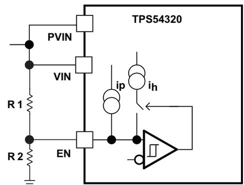
**Figure 19. Adjustable VIN and PVIN UVLO**
