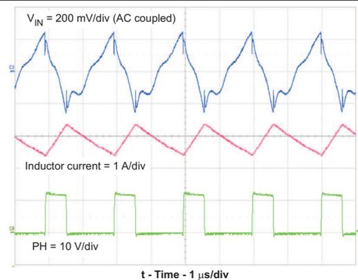
Figure 45. Input Voltage Ripple (1.1-Ω Load)
