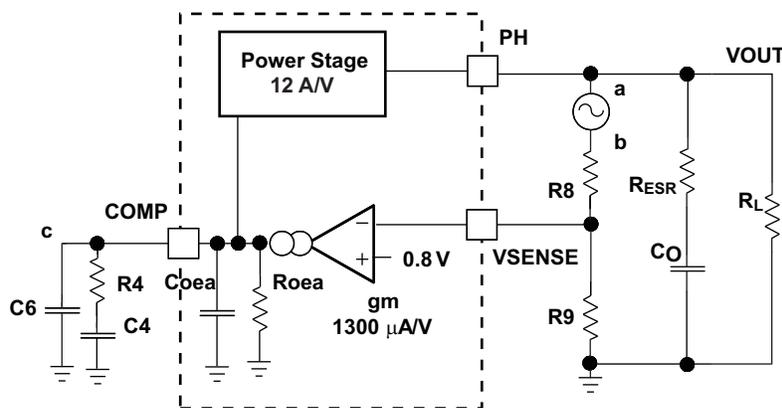
Figure 28. Small Signal Model for Loop Response
