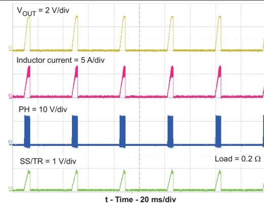
Figure 46. Overcurrent Hiccup Mode
