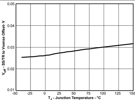
Figure 11. (SS/TR - VSENSE) Offset vs Temperature
