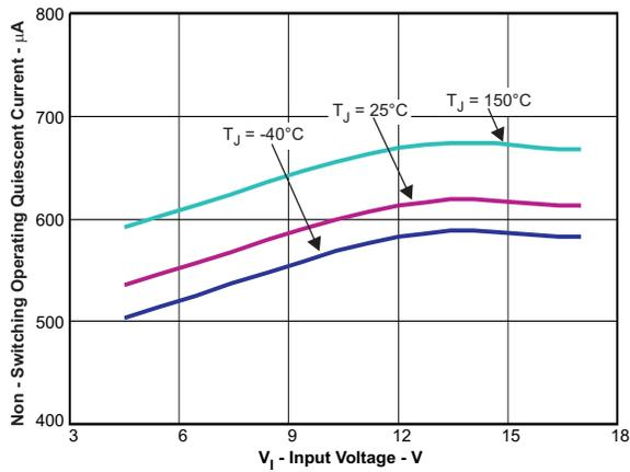
Figure 9. Non-Switching Operating Quiescent Current vs Input Voltage
