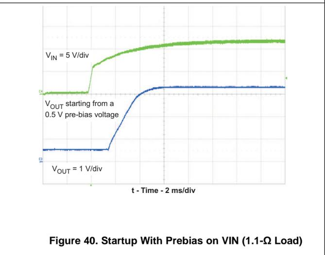
Figure 40. Startup With Prebias on VIN (1.1- $\Omega$  Load)
