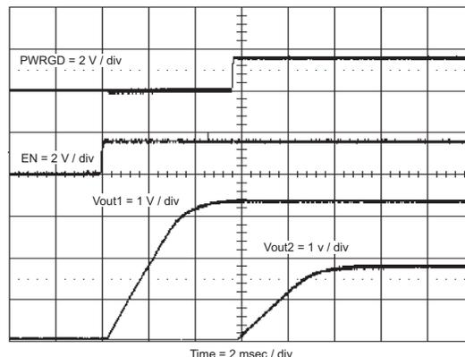
Figure 21. Sequential Start-Up Using EN and PWRGD
