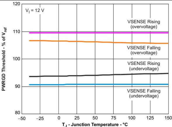
Figure 12. PWRGD Threshold vs Temperature
