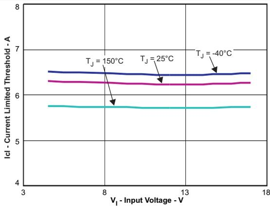
Figure 13. High-Side Current Limit Threshold vs Input Voltage
