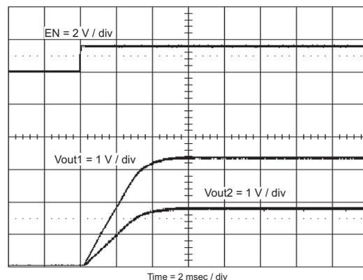
Figure 23. Ratiometric Startup Using Coupled SS/TR Pins
