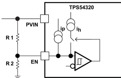
**Figure 18. Adjustable PVIN UVLO, VIN ≥ 4.5 V**
