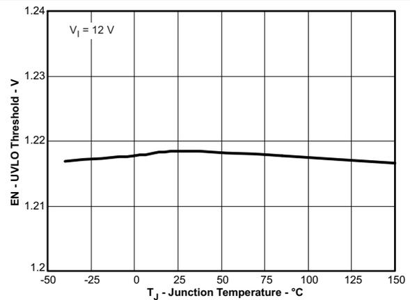
Figure 8. EN Pin UVLO Threshold vs Temperature
