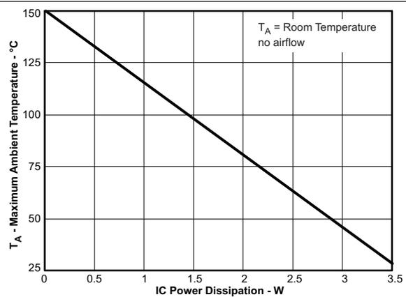
Figure 52. Maximum Ambient Temperature vs IC Power Dissipation
