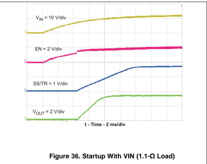
Figure 36. Startup With VIN (1.1- $\Omega$  Load)
