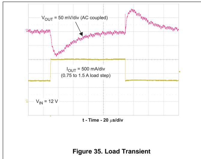
Figure 35. Load Transient
