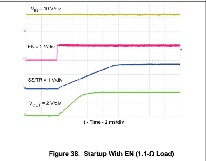
Figure 38. Startup With EN (1.1- $\Omega$  Load)
