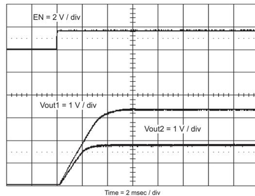
**Figure 25. Ratiometric Startup With Vout1 Leading Vout2**
