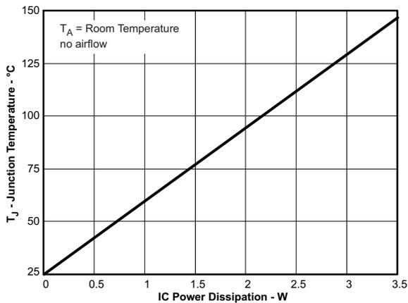
**Figure 53. Junction Temperature vs IC Power Dissipation**
