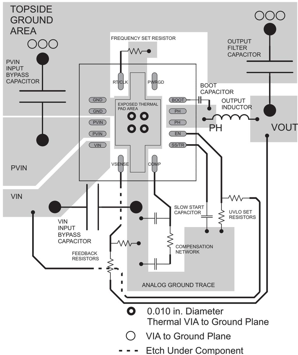
Figure 56. PCB Layout
