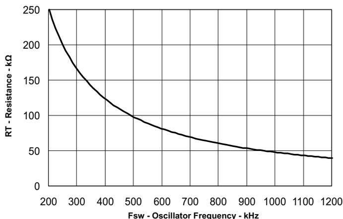
Figure 32. RT Set Resistor vs Switching Frequency
