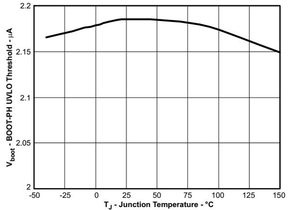
Figure 16. BOOT-PH UVLO Threshold vs Temperature
