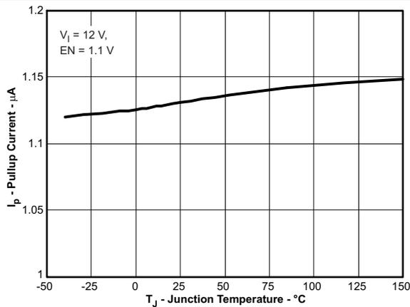
Figure 7. EN Pin Pullup Current vs Temperature
