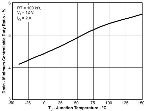
Figure 15. Minimum Controllable Duty Ratio vs Junction Temperature
