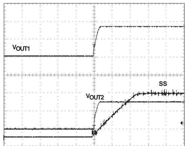
Figure 10. Start-Up Waveform
