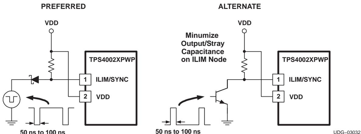
Figure 6. Synchronization Methods
